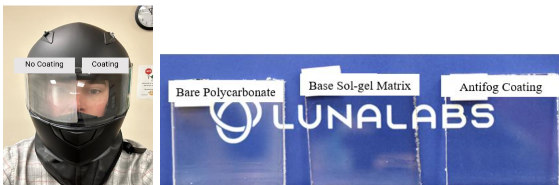
Figure 2. Representative pictures of Luna Labs' antifog coating: half of a motorcycle helmet visor (left) and on a cut polycarbonate substrate compared to bare polycarbonate and the base sol-gel matrix.
