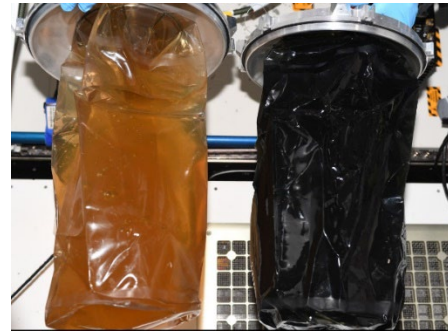
Figure 11. Comparison of UWMS filled EDV (Russian tank) and WHC previously filled EDV. Tank on left contains UWMS urine and does not appear to contain pretreat. Tank on right is a previously filled tank used on WHC (Waste and Hygiene Compartment.)
