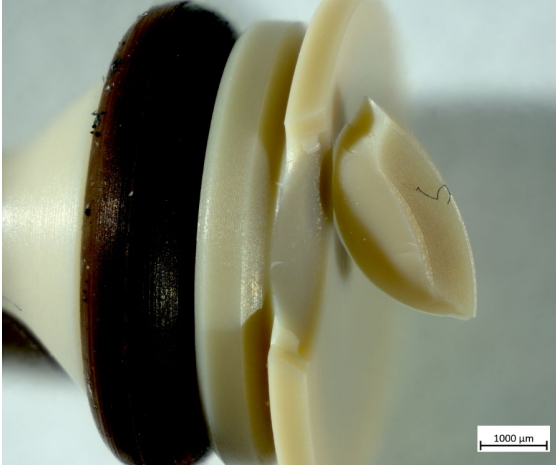
Figure 16. Poppet with broken piece
