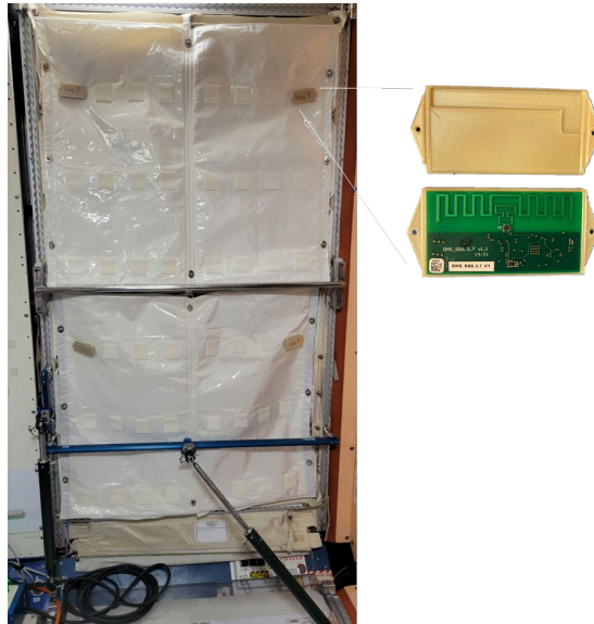
Figure 8. Four DMS tags on NOD1S4 ZSR doors in Space Vehicle Mockup Facility at JSC.
