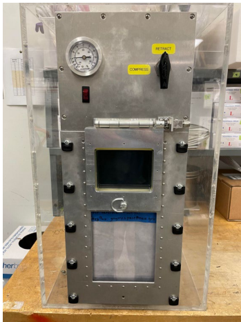
Figure 14. Laboratory Benchtop Trash Compaction Test System.
