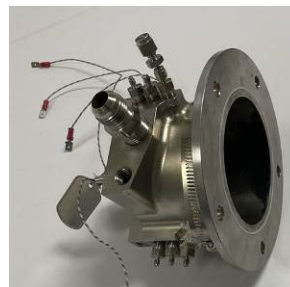
Figure 15. Subscale Trash to Gas OSCAR reactor.
