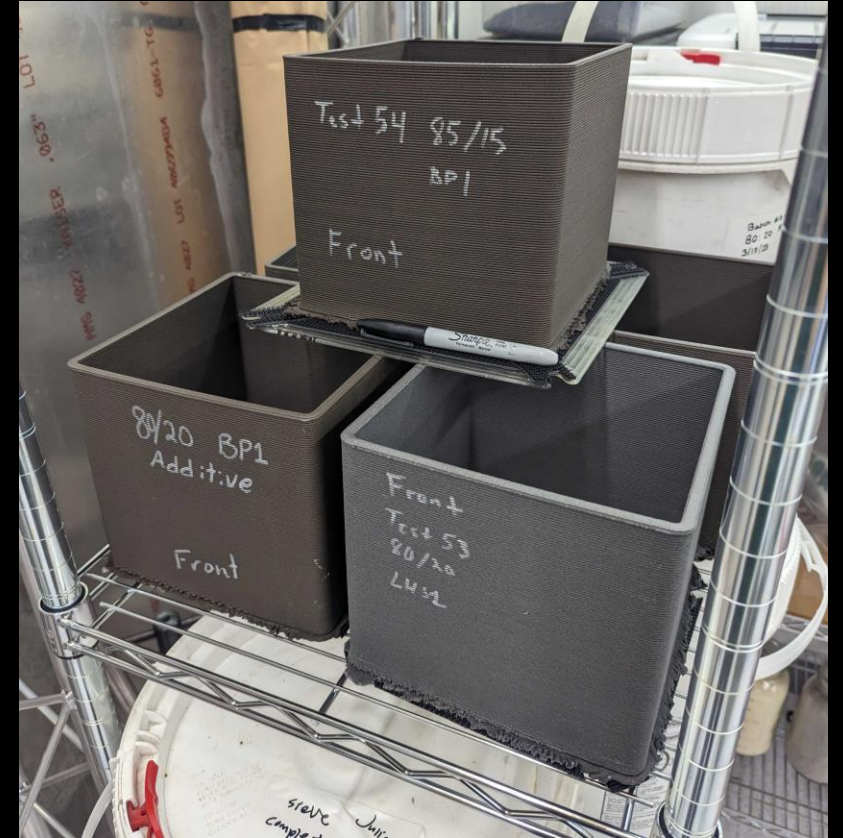
Printed test samples prior to water-jetting
