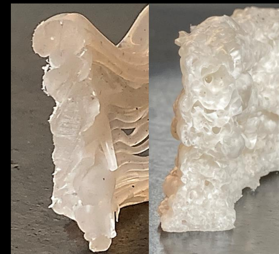
A compatibilizer additive contributed to porosity
