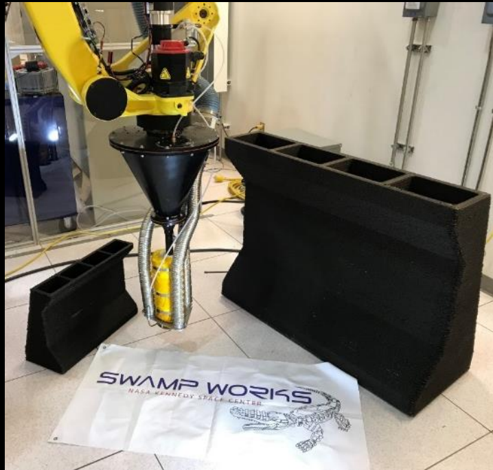
A partnership with Autodesk develops toolpath algorithms and 3D prints barricades/blast walls
