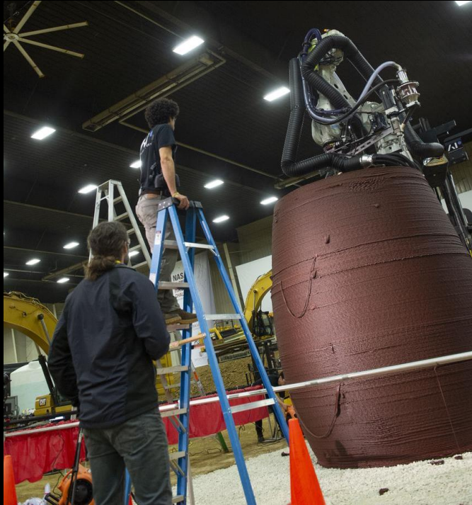
AI Space Factory 3D prints a polymer-basalt fiber habitat prototype*
