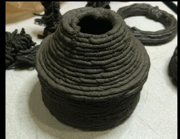
First RPC structure is printed showing feasibility
