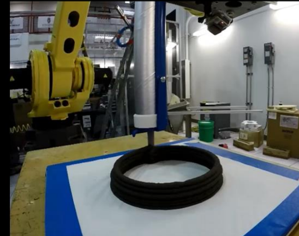
Extrusion of premixed silicone and regolith
