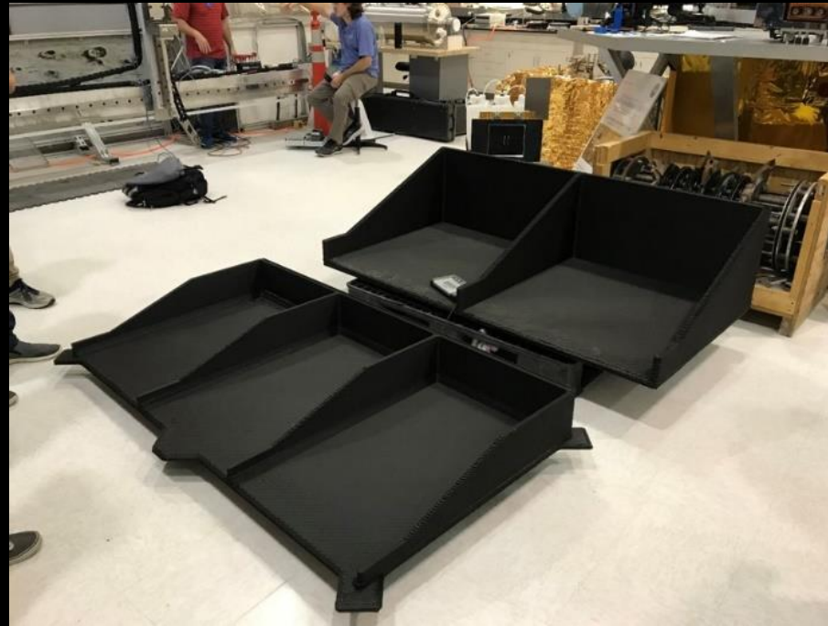
A partnership with NASA's Exploration Ground Systems Project produces 3D printed concrete formwork
