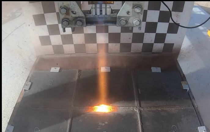
Paver grouting mitigates plume effects
