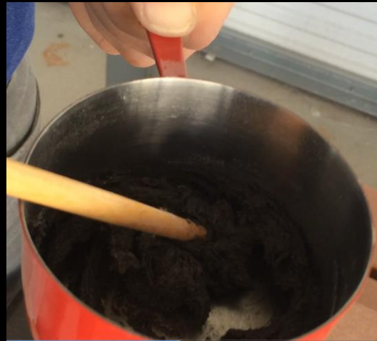
Mixing regolith and plastic while hot shows promise
