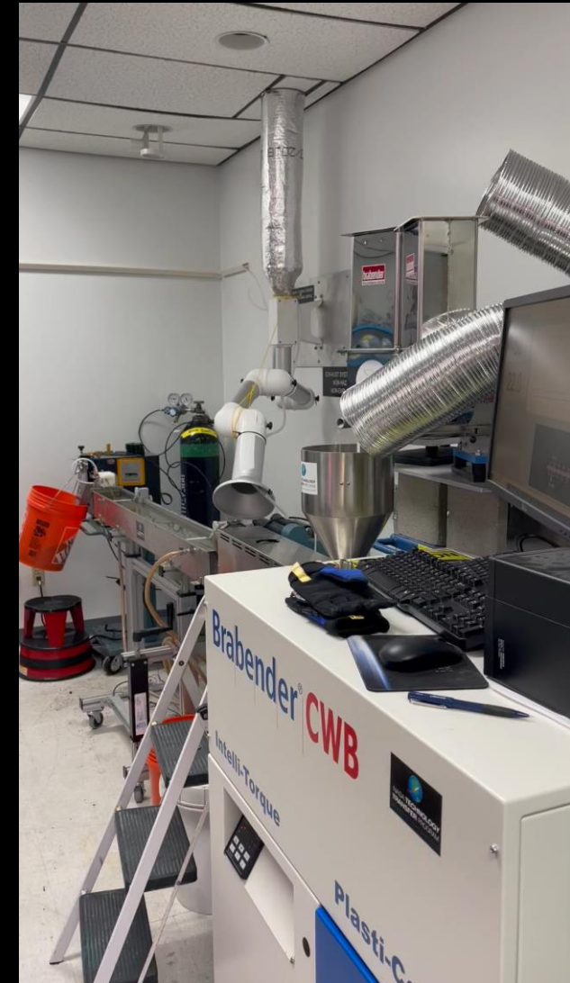
RPC pellets are produced on a compounding extruder
