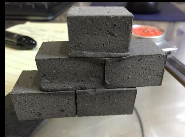
RPC blocks are adhered by remelting adjacent surfaces
