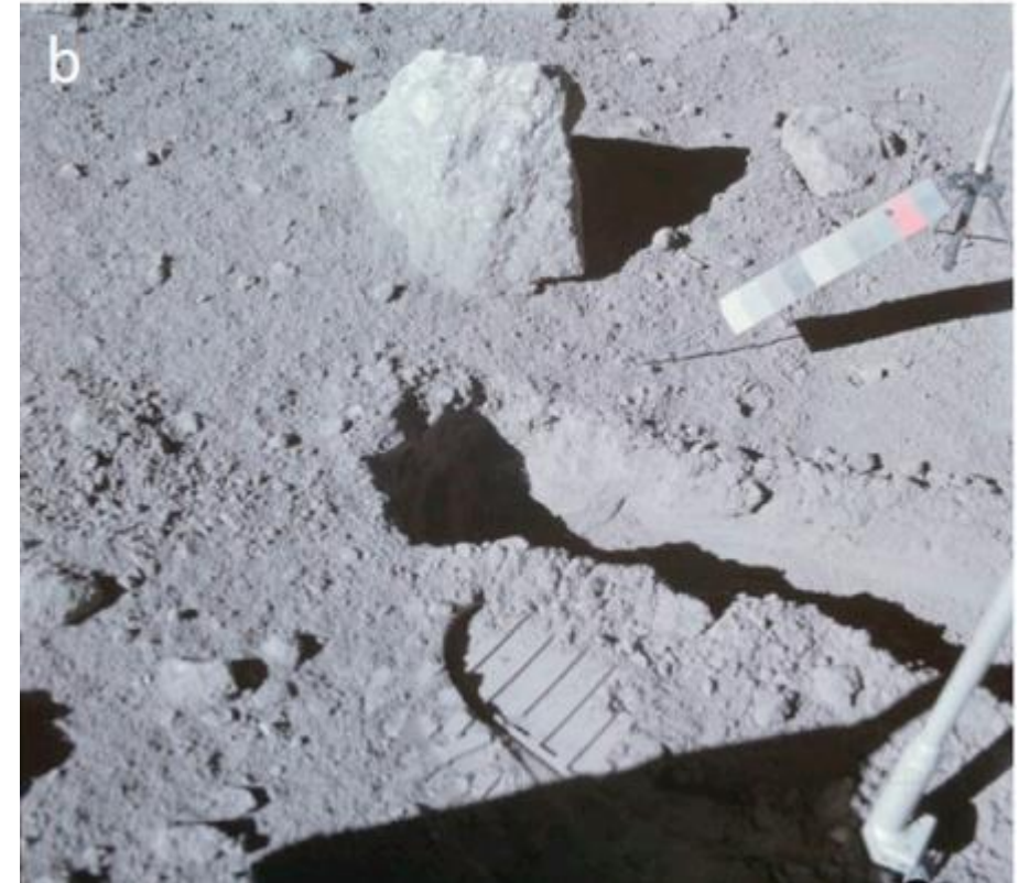
Trench dug during the Apollo 16 mission showing the cohesive behaviour of lunar soil. Astronaut boot print for scale (Credit: NASA AS16-107-17458).
