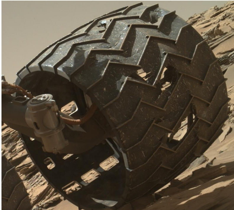
Curiosity's wheel with premature damage
