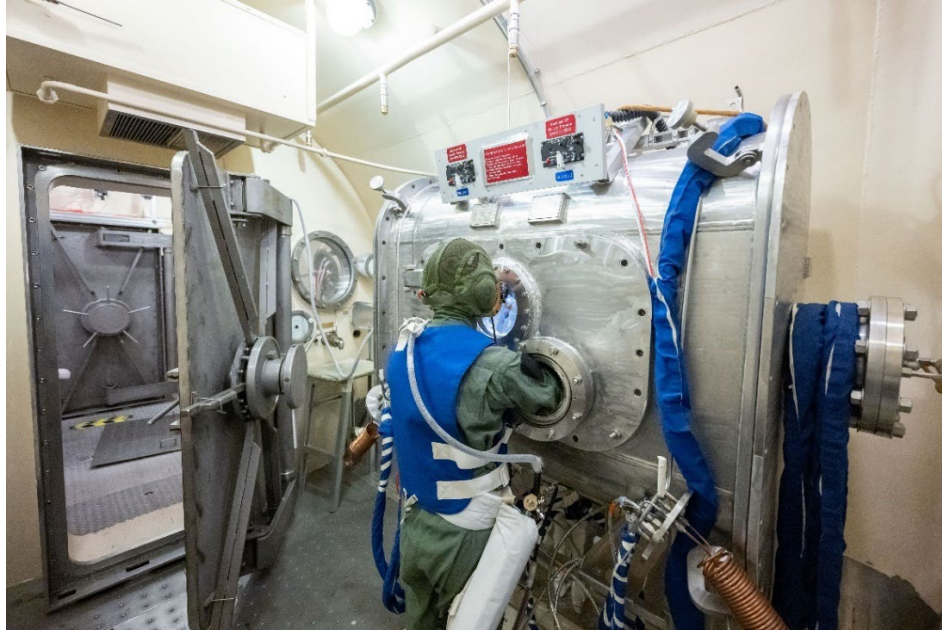
Figure 5. Test subject within the 11-foot chamber and operating hardware with EMU gloves in the DGB.
