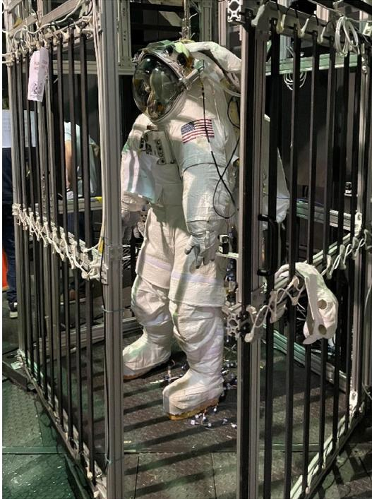
**Figure 2. Suit 2 Test Article, Inside Heater Cage.**
