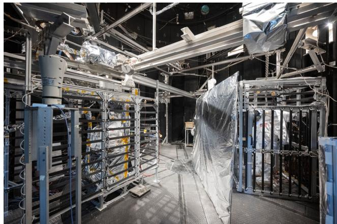
**Figure 15. Mylar divider between the test articles.**
