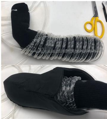
Figure 4. Foot Simulator (Top), Foot Simulator in BSI (Bottom).
