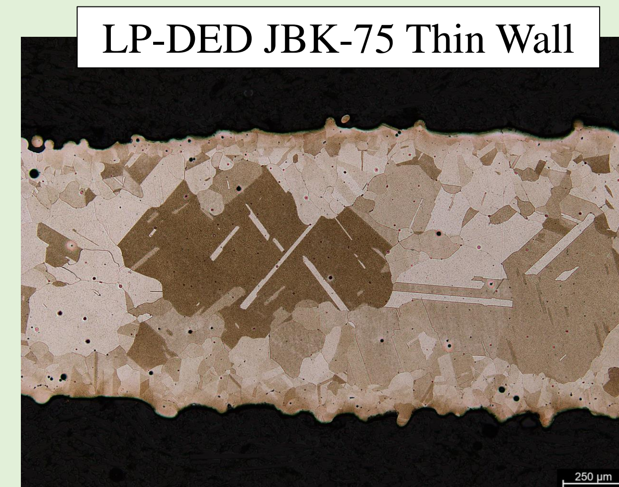
Large Seeded Defect Post HT
