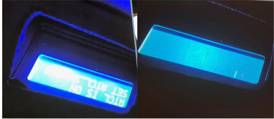
Figure 3. DCU LCD screen in ambient (Left) and cold (Right) environments.
