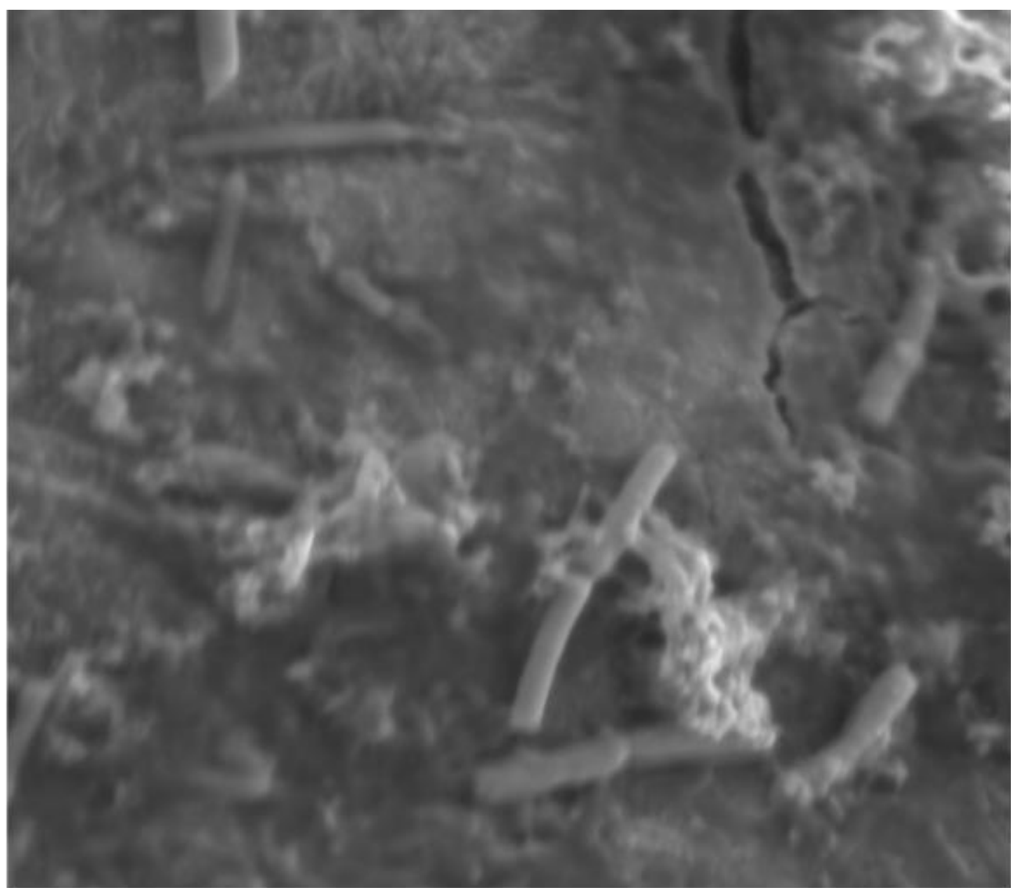
Microbes on Additively Manufactured Copper, Imaged on FEI ESEM, 7kx
