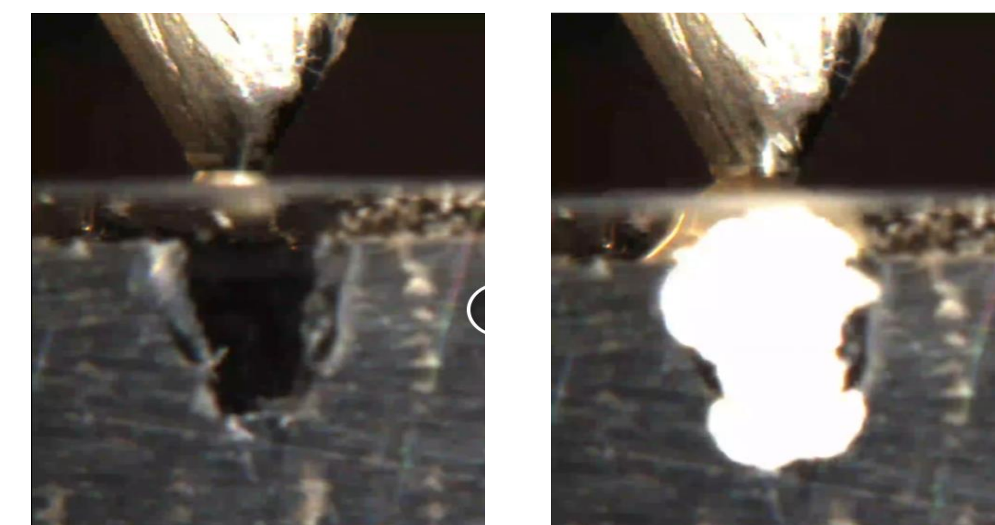
Parabolic flight via-filling experiment with conductive silver ink.
