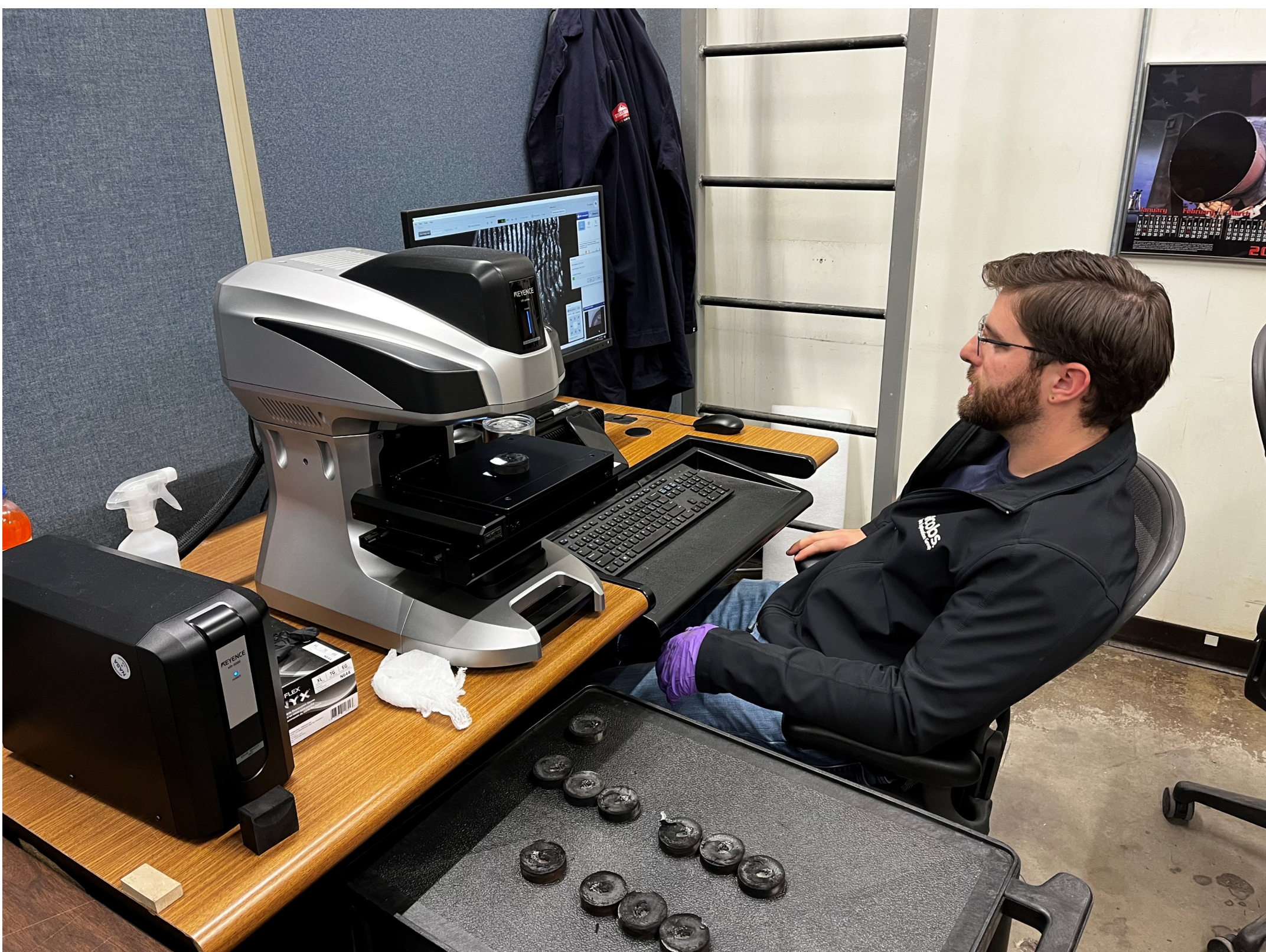
Caption: A technician scans post test plasma torch specimens
