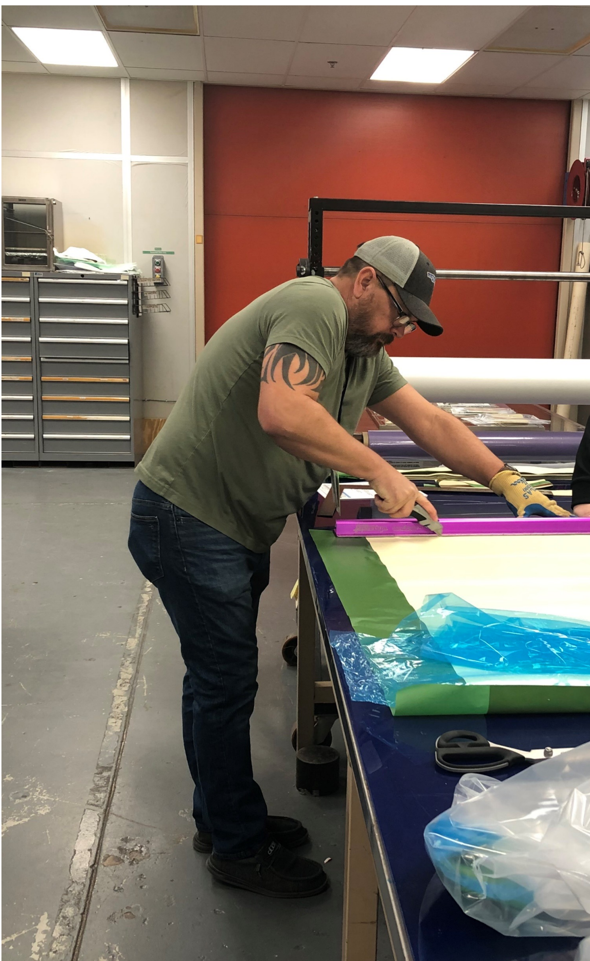
Caption: Technician cuts rubber for specimen layup
