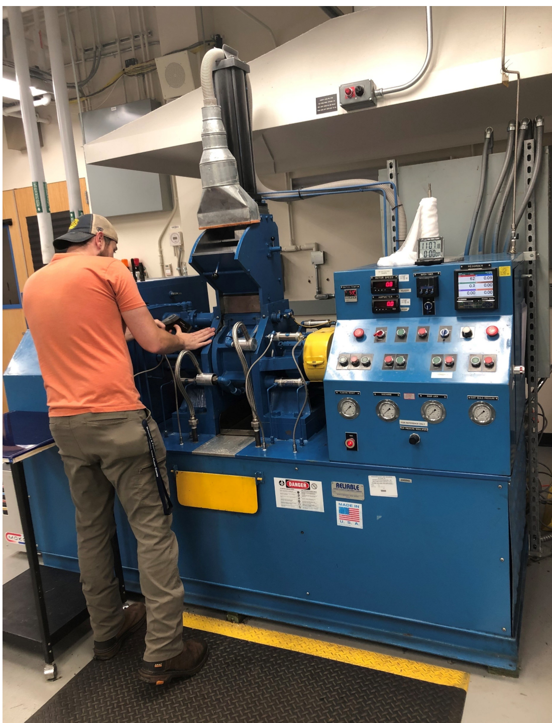
Caption: A technician checks the temperature of the mixer seals during mixing
