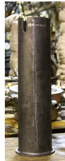
SiC/SiC Combustor Liners: Outer Liner and EBC Coated Inner Liner
