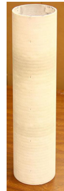
SiC/SiC Combustor Liners: Outer Liner and EBC Coated Inner Liner
