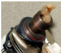
Figure 2: Biofilm accumulation in piping 2
