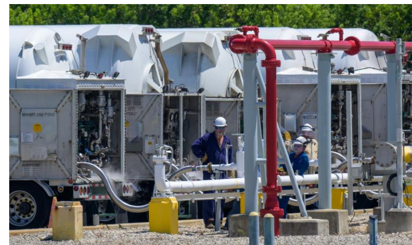
Tanker trucks deliver liquid hydrogen (LH2) to replenish the large sphere at NASA's Kennedy Space Center in Florida, Launch Pad 39B. (NASA Image NHQ202208310013)
