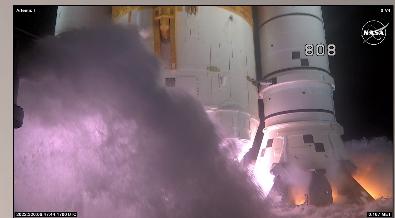
Ignition Overpressure Protection and Sound Suppression System
