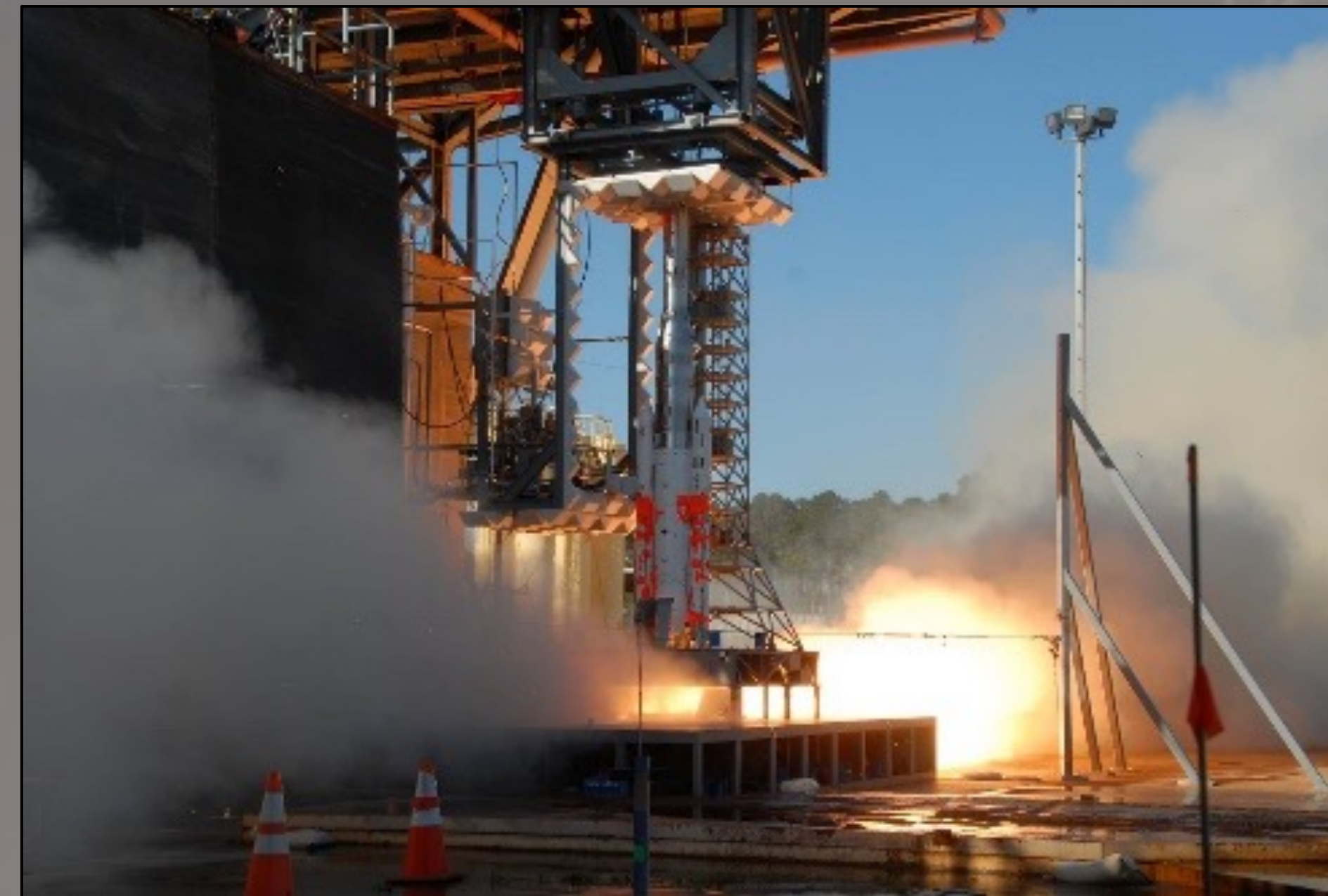
SLS Subscale Model Acoustic Test
