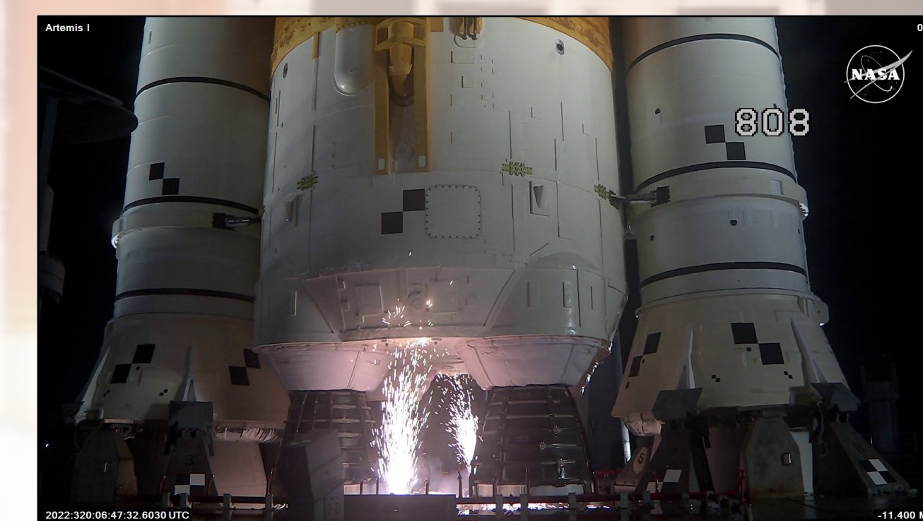
Hydrogen Burn-Off Igniters during SLS Hold-Down
