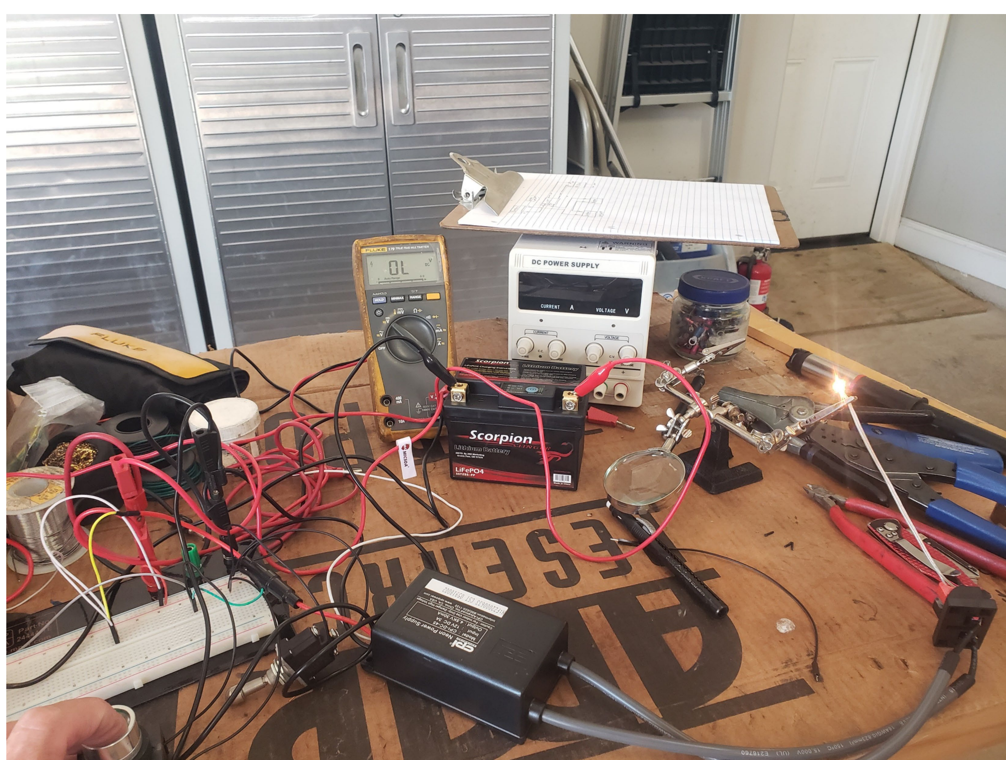
Electrical Circuit / Igniter System
