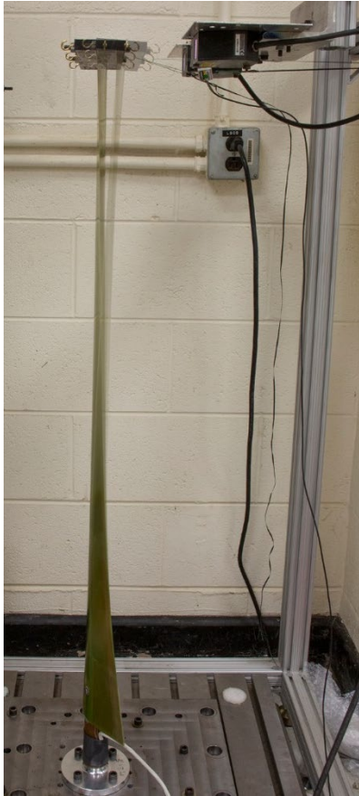
Figure 12. Static loading of a rotor blade.
