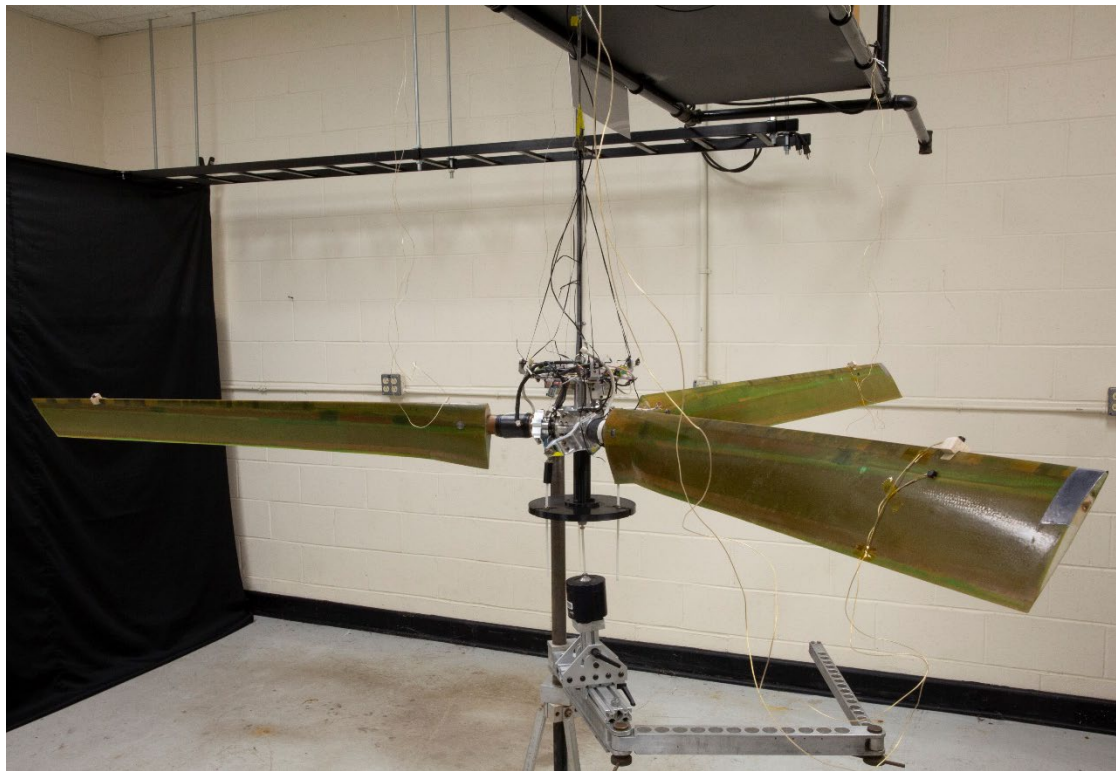
Figure 13. Free-free rotor test with the shaker setup.
