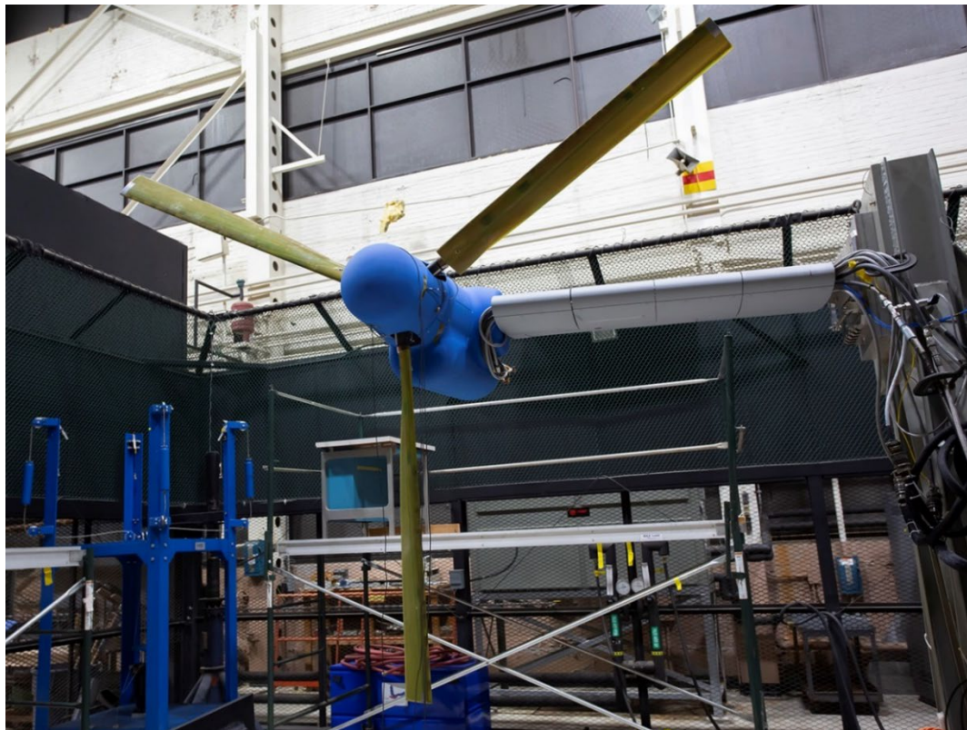
Figure 21. TRAST hover cell GVT with blades installed.
