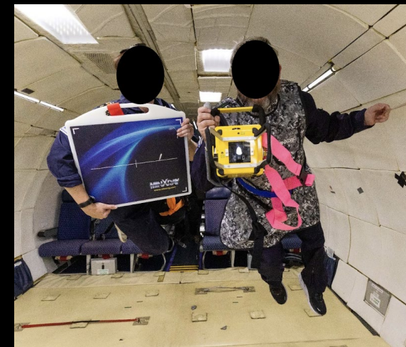
Above top: Handheld radiography system Above bottom: Portable radiography equipment in parabolic flight
