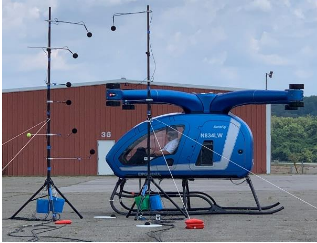
Fig. 7 The microphone array used for the electric motor noise measurements.
