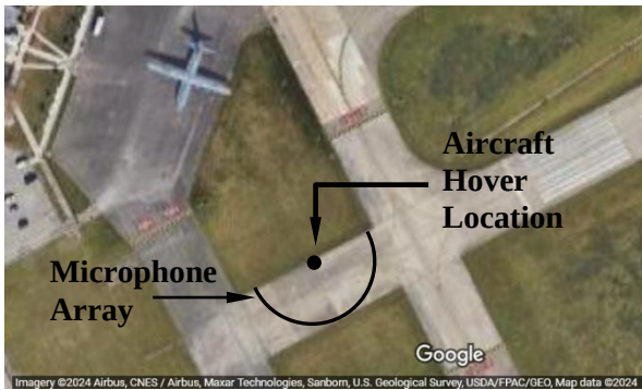
Fig. 3 The aircraft position and microphone array locations used in Hover Test 1 at Lunken Municipal Airport.
