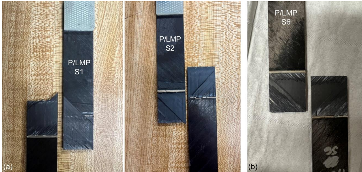
Figure 7. Broken SLS joints using LM-PAEK interlayer with hybrid PEEK/LM-PAEK adherend. (a) At RT. (b) At ET.
