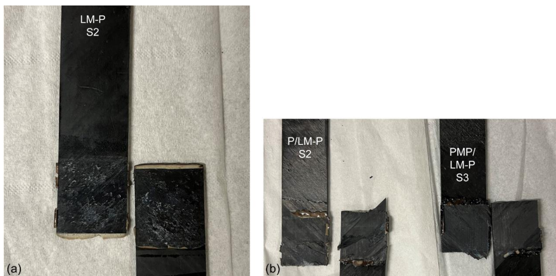
Figure 11. Broken SLS joints using LM-PAEK interlayer at RT. (a) PEEK adherends with LM-PAEK interlayer. (b) Hybrid PEEK/LM-PAEK adherends with LM-PAEK interlayer.
