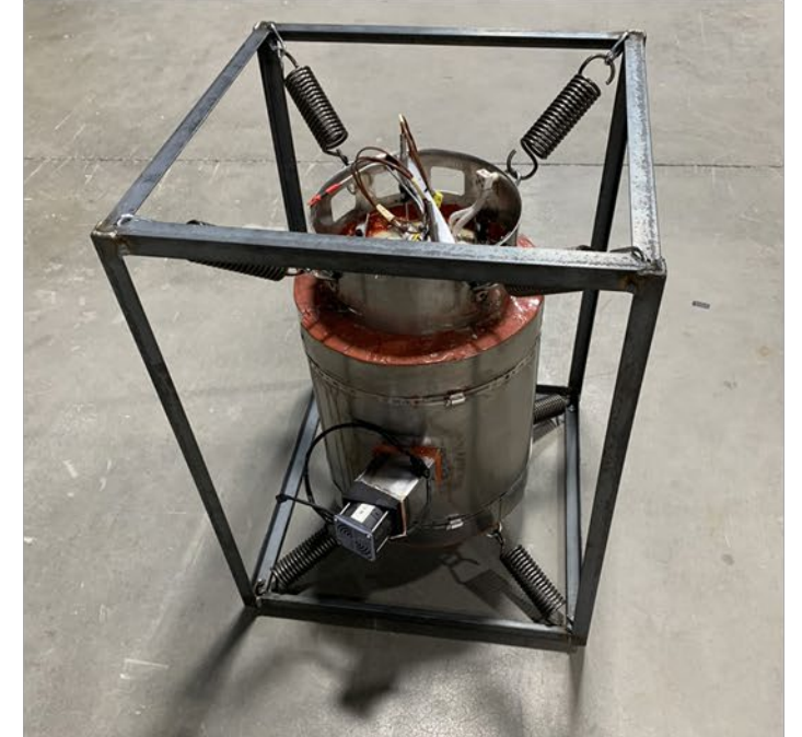
M-COG Oxygen Engine Cell stack, heater, heat exchanger, blower, structure, packaging for transport. The hot part of the system
