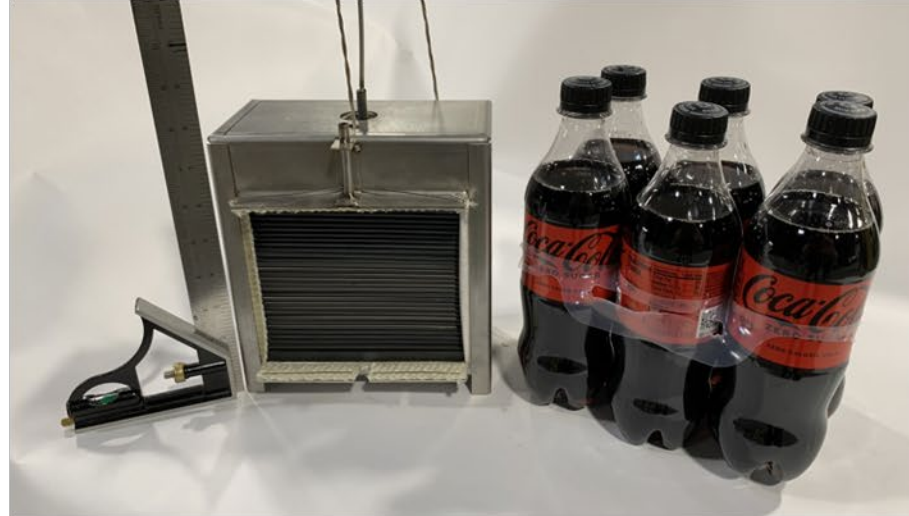
M-COG cell stack 8" X 8" X 4". 30 wafers, joined together into a single system, with thermal and electrical isolation - in a stainless steel housing for modular installation. Each cell stack produces about 4 lpm oxygen.
