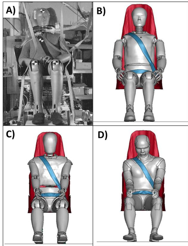
**Figure 3: Tested ATD initial position (A) and model positions for Hybrid III (B) THOR (C) and GHBMC (D).**
