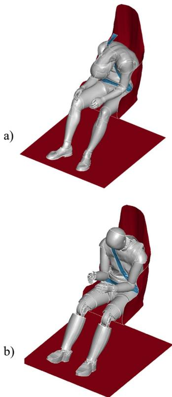
**Figure 8: Test 3 occupant deformation at 200 ms: GHBMC (a) and THOR (b).**
