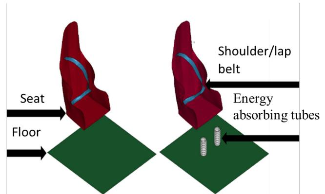
**Figure 1. Seat models for the standard seat (Left) and energy absorbing (EA) seat (Right).**
