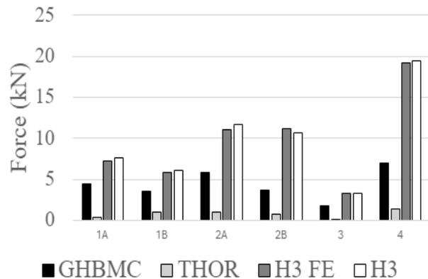
**Figure 9: Lumbar force for each test condition.**
