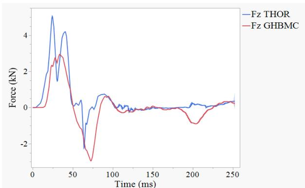
Figure 6: Vertical force for GHBMC and THOR in test 4.
