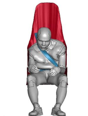
**Figure 10: Abdominal compression of GHBMC model in test 4 test condition.**
