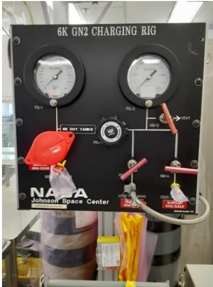
Figure 2. 6K GN 2 charging rig photo. The 6K GN 2 charging rig provides nitrogen gas stored in four tanks as well as pressure control valves and gauges to supply the SxEMU O 2 tanks with 3,000 psi gas.
