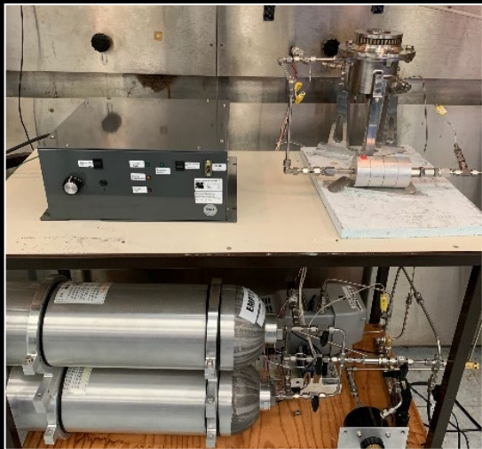
HEOMD AES – Logistics Reduction Trash Venting. Left: Plasma gasification/pyrolysis reactor; Right: OSCAR combustion/gasification/incineration Trash to Gas test rig.
