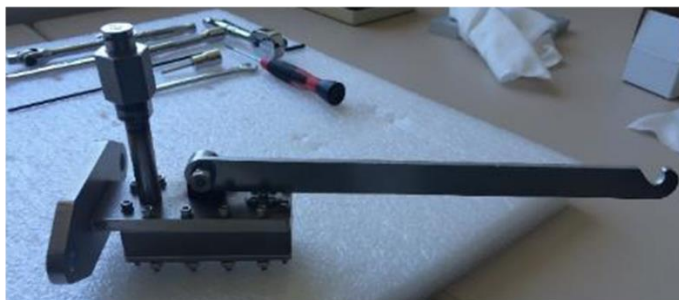
NASA Designed Loading Fixture for Exposure to LMP-103S Propellant – NASA New Technology Report (1461267027)
