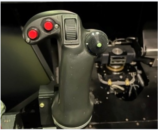
Left Stick with Hover Engage/Disengage Buttons
