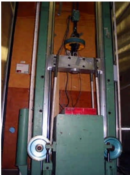
Drop tower capable of 100/s strain rate
