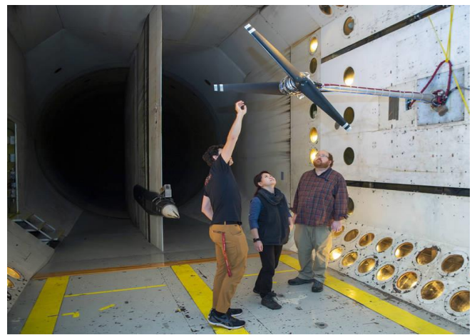
Figure 4. NASA LaRC Transonic Dynamics Tunnel Test, Dragonfly Phase B* Coaxial Rotor System.
