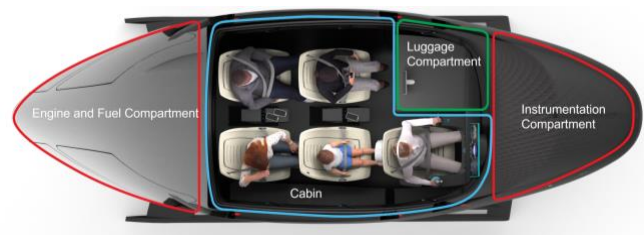
Figure 7. Top view of 5 occupant quadrotor cabin layout
