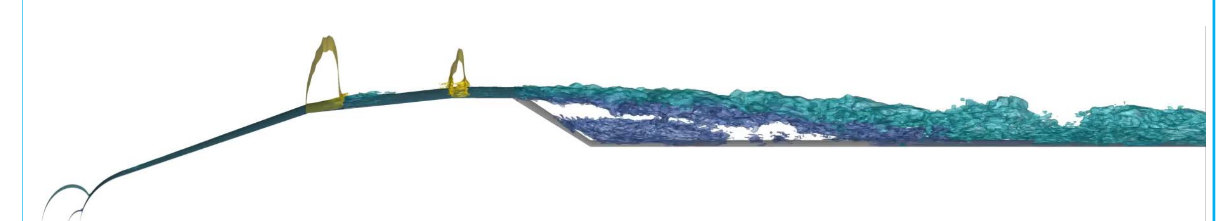
Caption: Iso-surfaces of Mach number from a M=0.8 simulation conducted with HRLES on the Coe hammerhead geometry.
