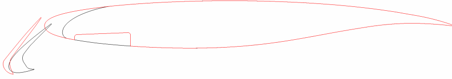
Fig.1 Computational airfoil geometries. Black: configuration with a conventional slat, red: configuration with a Krueger flap with an exposed cavity.
