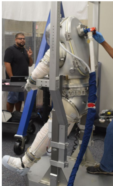
Figure 4. Pike position with straight legs to evaluate leg length, hip indexing, and shoulder straps.
