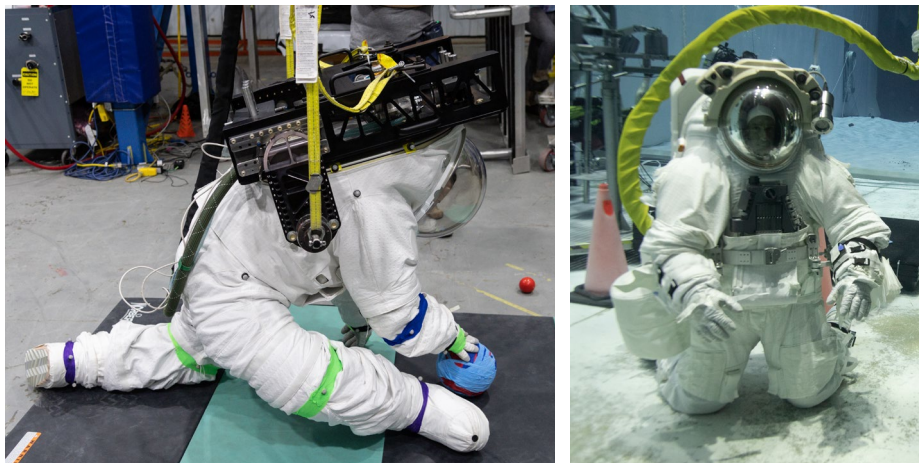
Figure 8. Subjects performing mobility tasks in different environments to establish acceptable fit. Test facility: ARGOS (left) and NBL (right).
