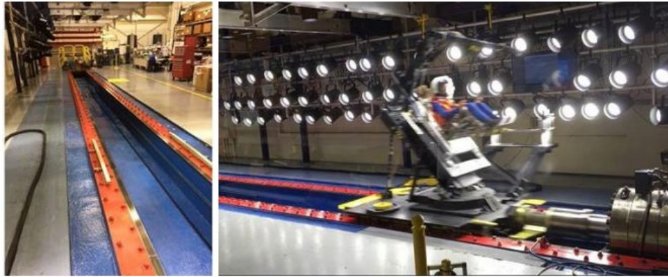
Figure 1. The horizontal impact accelerator (HIA) at Wright-Patterson Air Force Base. The photo on the left shows the sled track, and the photo on the right shows an ATD suited test [4].
