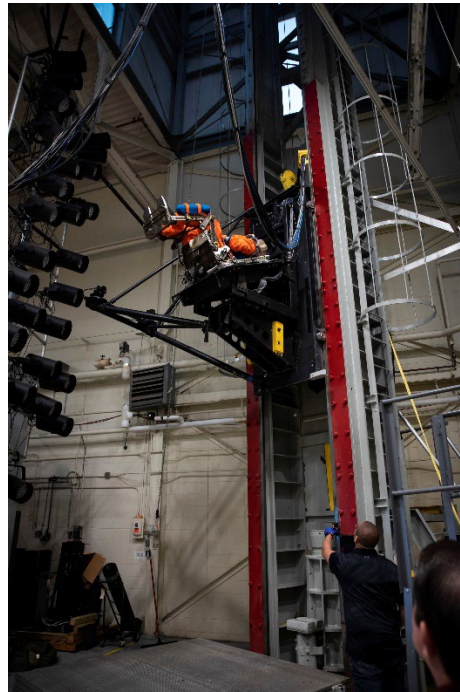
Figure 2. The vertical deceleration tower (VDT) at Wright-Patterson Air Force Base. The photo shows a human subject being raised to the required drop height [5].
