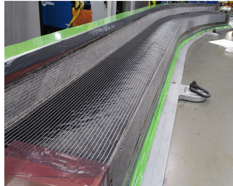
Saertex Triaxial NCF Formed on a Curved Z Geometry
