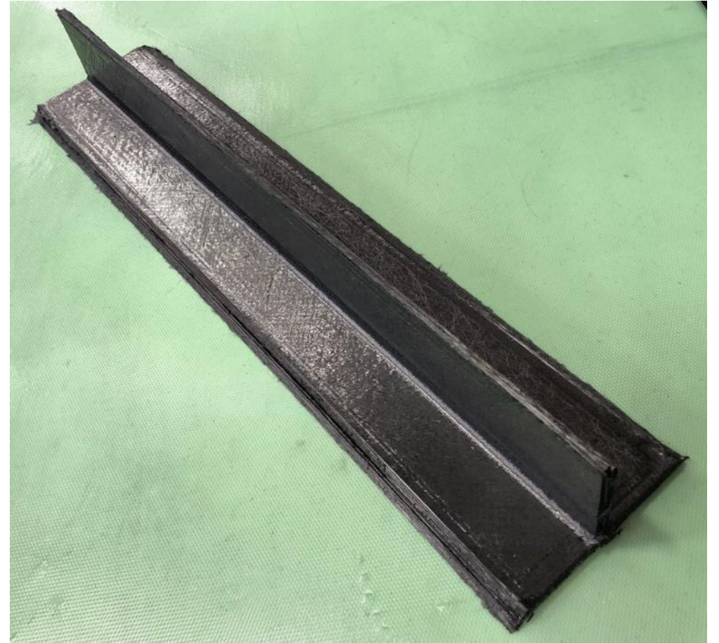
T-Stringer Preform Made from Quad NCF
