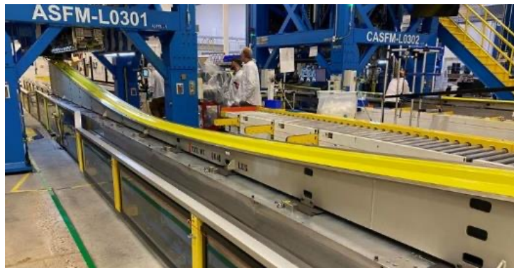
ASFM Used for Production Thermoset Stringers
