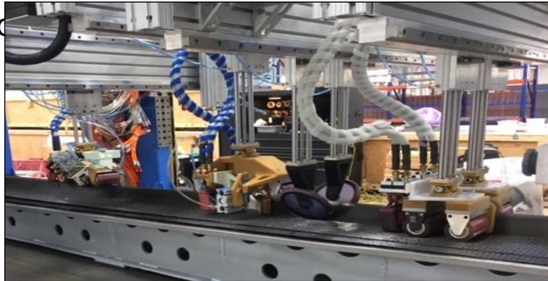
ASF Progressive Forming of an NCF Omega Stringer
