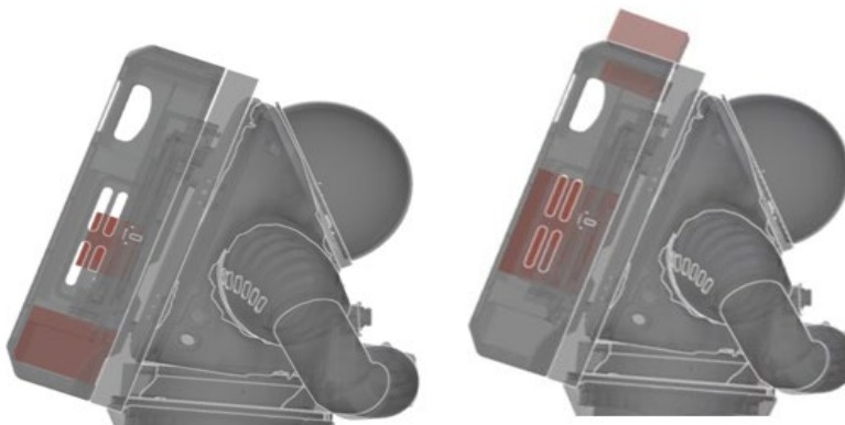
Figure 3. Left: 2022 NBL series foam locations (red 3highlighted boxes). Right: 2023 NBL series foam locations.
