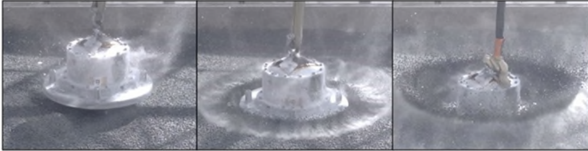
Figure 15. High speed photographs of test vehicle containing sleeves, RSTAs, and crushable lattice impacting the gravel bed.
