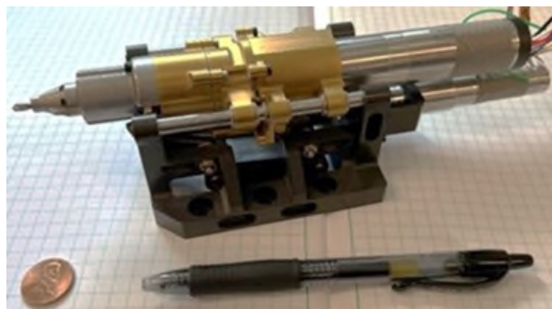
Figure 1. Image of the Micro-Sampler with items shown for scale. This assembly weighs 0.9 kg.
