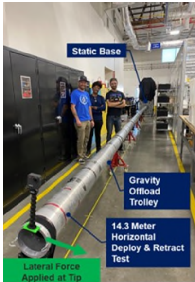
Figure 15. DIABLO boom demonstrating properties of mechanical slop and ideal beam. A lateral force is applied to the tip of the mast while the base is held static. It is swept across the deployment axis, where left is negative lateral deflection and right is positive lateral deflection.
