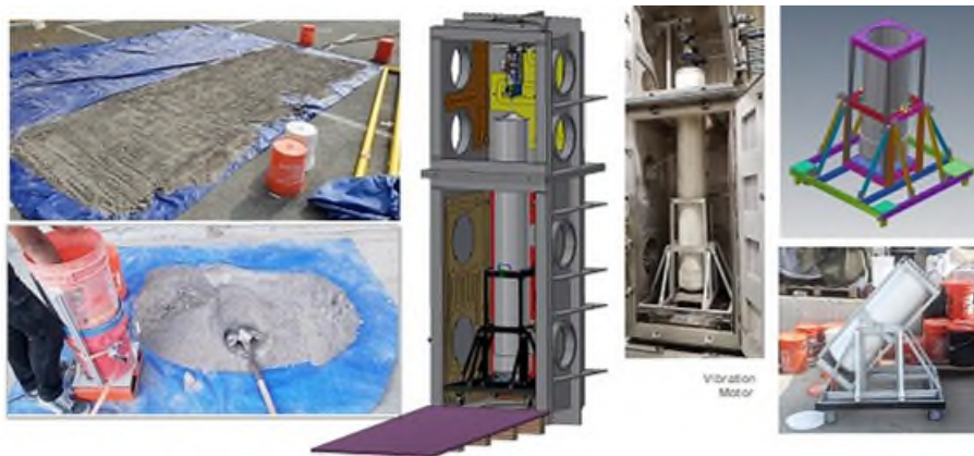
Figure 18. Regolith analog BP-1 used to test DIABLO-based pneumatic drill science instrument. A large regolith bin with a vibration motor is used to vibrate-compact the regolith.
