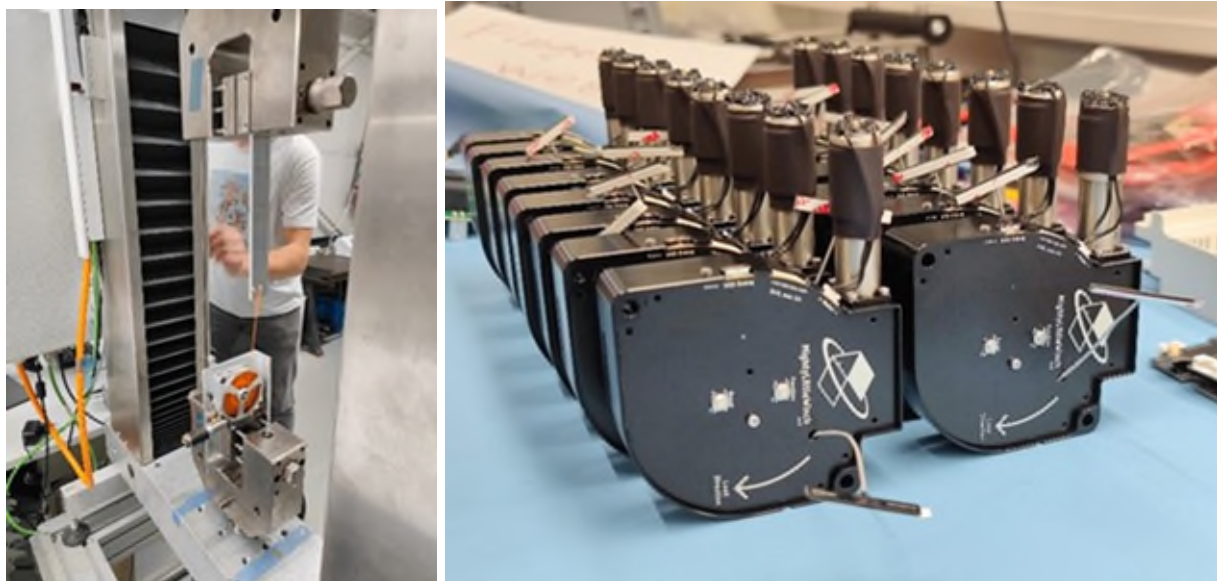
Figure 3: Micro winch prototype during tension-loading test (left). Following validation of the prototype, a batch of micro-winches was manufactured and prepared for integration (right).
