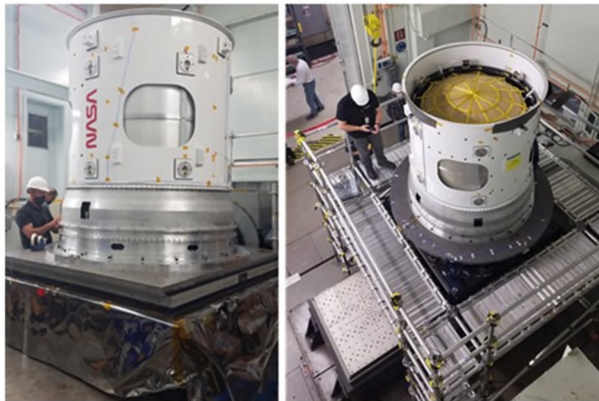
Figure 16 PASS random vibration testing - lateral (left) and axial (right).
