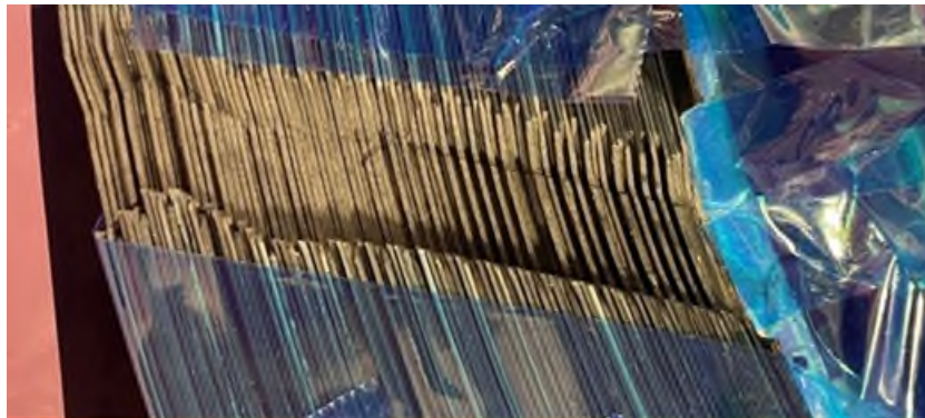
Figure 11. Notch migration due to inner flange buckling, prior to second notch cutting process.
