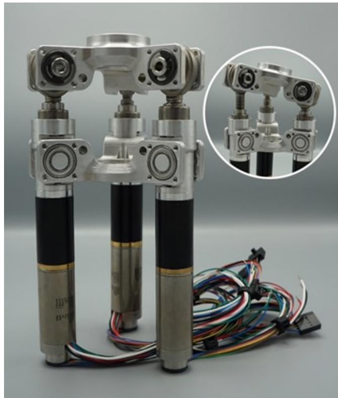
Figure 1 - Programmable Lead Screw Actuated Self-Leveling Platform (PLSASLP) in standby position; detail on the right shows the PLSASLP tilted at 10 degrees. Prototype is complete and undergoing testing.
