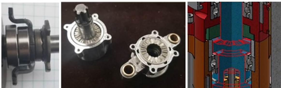
Figure 4. (left) Sawtooth dog elements extracted from a commercial drill machine. (center) Image of the lobed dog clutch in the percussor housing. The dog element on the left rotates with the drill string shown in blue in the CAD section view (right). The upper dog (green) is constrained by the percussor housings (orange and red).
