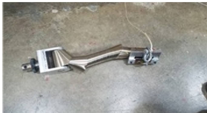
Figure 10 PASS CF Spring Failure
