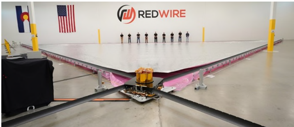
Figure 1. Solar Cruiser TRL 6 prototype following single quadrant deployment testing.
