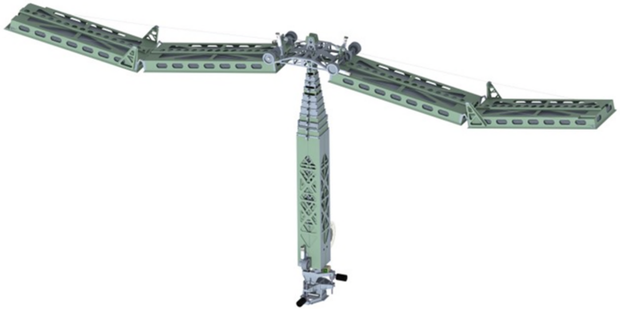
Figure 15. Four Array Configuration at “Kicker” Contact Deployment Stage
