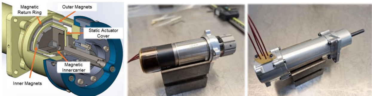
Figure 5. Magnetic coupling design and drive sub-system 'in-progress' images: Actuator test-fit with magnetic coupling inner (left), non-redundant actuator mounted in sealed housing (center), motor in sealed housing with drive wheel spigot (right)
