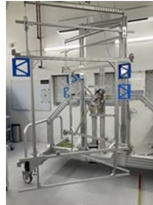
Figure 11. Breadboard SAW for Synchronization Cable characterization (Yoke + 2 panel configuration)
