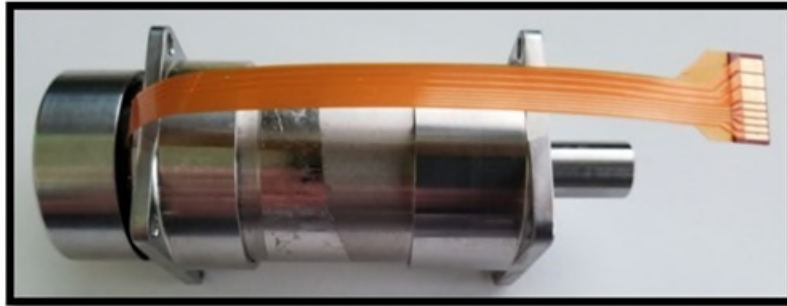
Figure 6. BMG Planetary Gearmotor EDU consisting of a COTS size 32 Maxon motor integrated with the 166:1 PoC design BMG planetary gearbox.
