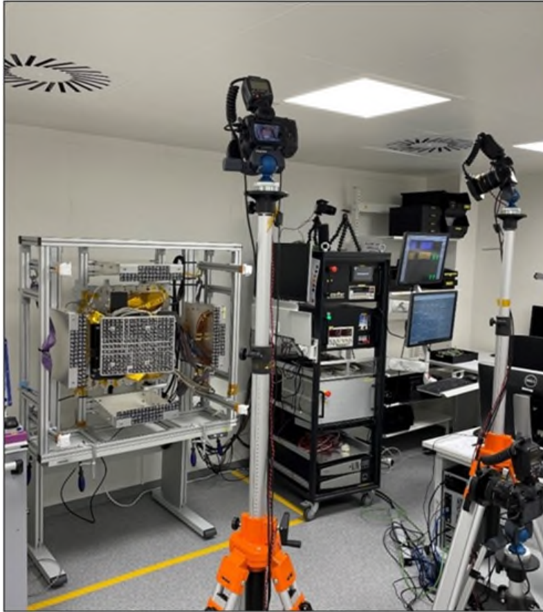
Figure 14. Pointing Performance Test Setup at BGA (shown for X direction)
