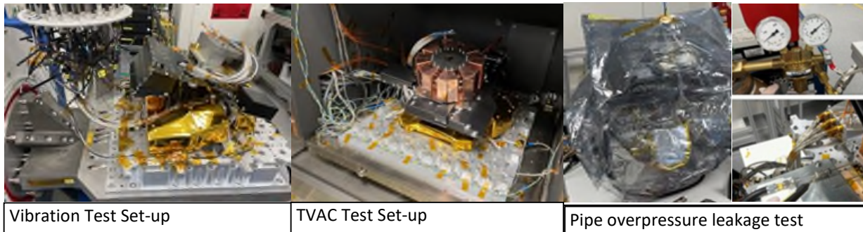
Figure 13. Vibration, TVAC, and Pipe Overpressure He Leakage Testing
