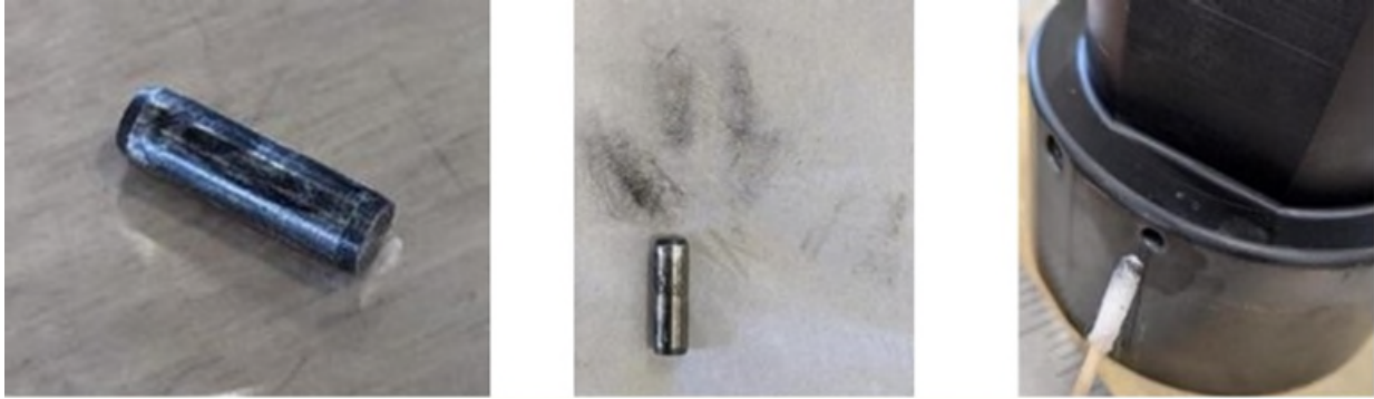
Figure 18. Lubricant on Pin (Left). Lubricant Wiped (Center). Lubricant in Hole (Right)
