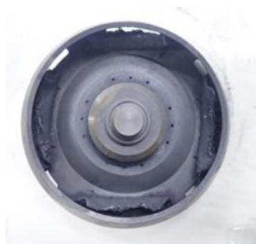
Figure 12. Powder bags attached to the lift cone
