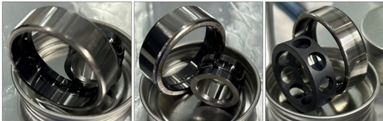
Figure 13: Images showing new bearings with HPS-2832 coating on raceways, and a custom PGM-HT cage with a hole-slot-hole ball pocket configuration prior to assembly
