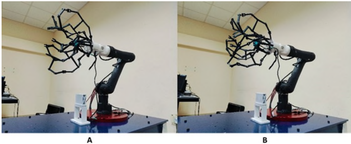
Figure 13. Robotic arm with engulfing end-effector (A) Open condition (B) Closed condition
