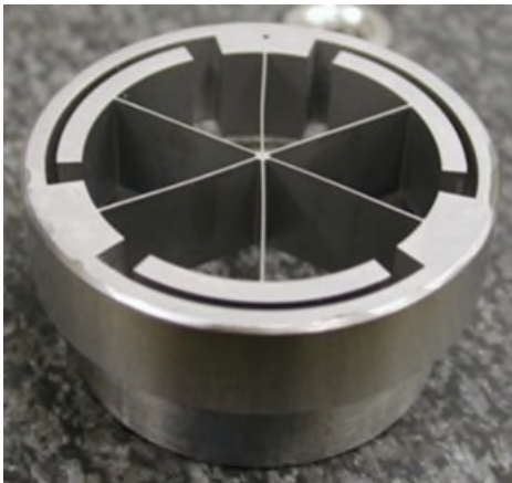
Figure 13. A pivot flexure with minimized center shift and integral travel limits.
