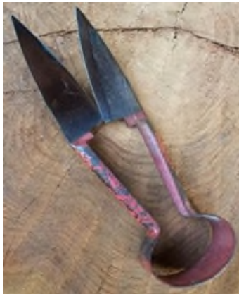
Figure 1. My grandfather's vintage sheep shears. This was made from a single sheet of steel which was cut, bent, and folded as needed to produce the blades, handles, and flexure.
