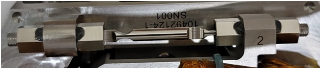
Figure 17. A flexured rod that makes up part of a precision mount assembly commonly used at JPL on opto-mechanical devices. It is referred to as a “Moore Mount” after its originator, Don Moore. These were machined using an end mill.
