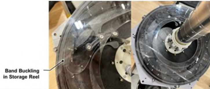
Figure 13. Band buckling failure more inside Storage Reel during retraction.
