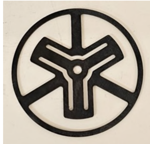
Figure 9. My very first flexure design. Versions of this diaphragm flexure design were cut by wire EDM and by milling.
