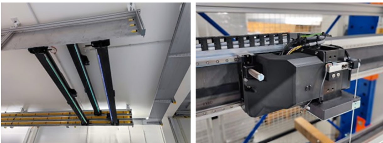
Figure 16: Latest version of the traverses with LED indicators visible running along the lower edge (left). Detail of a micro-winch with force sensor on the offloading cord (right).
