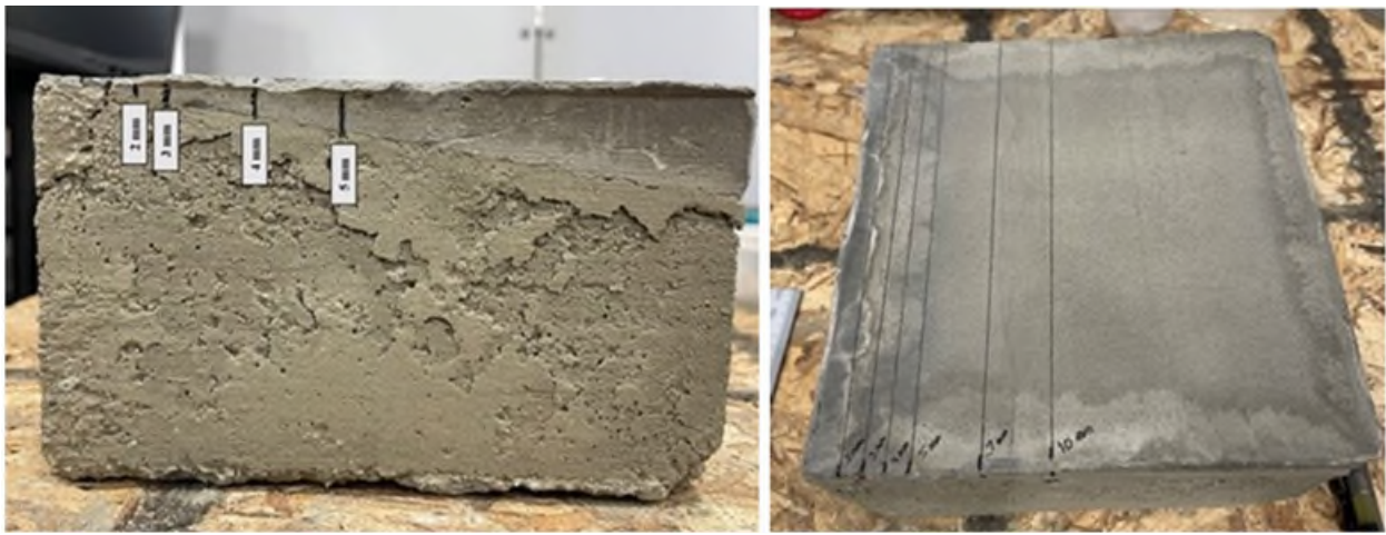
Figure 15. Different overburden layers shown on side profile of test media (left) and test media overhead view (right). The Micro-Sampler was used to drill holes and collect powder along the demarked lines. Controls were taken from the right side of the block, drilling only into overburden.
