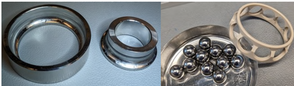
Figure 9. Bearing Cage and Balls Post Vibration Testing
