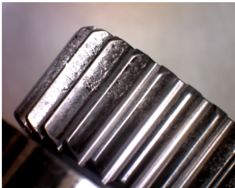
Figure 7. Damage to Last Stage Gear Mesh
