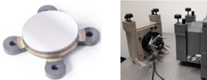
Figure 4: Free state mirror (left) and Mirrors RWE test after integration (right)
