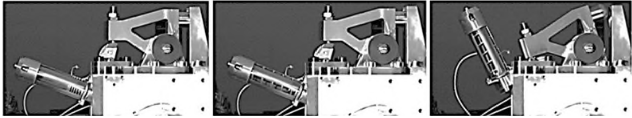
Figure 10. RM BB release test sequence: SNA actuation (left), bolt impact (center) and latch impact (right)
