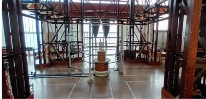
Figure 4: Magnetic moment measurement on EM1 (CNES)
