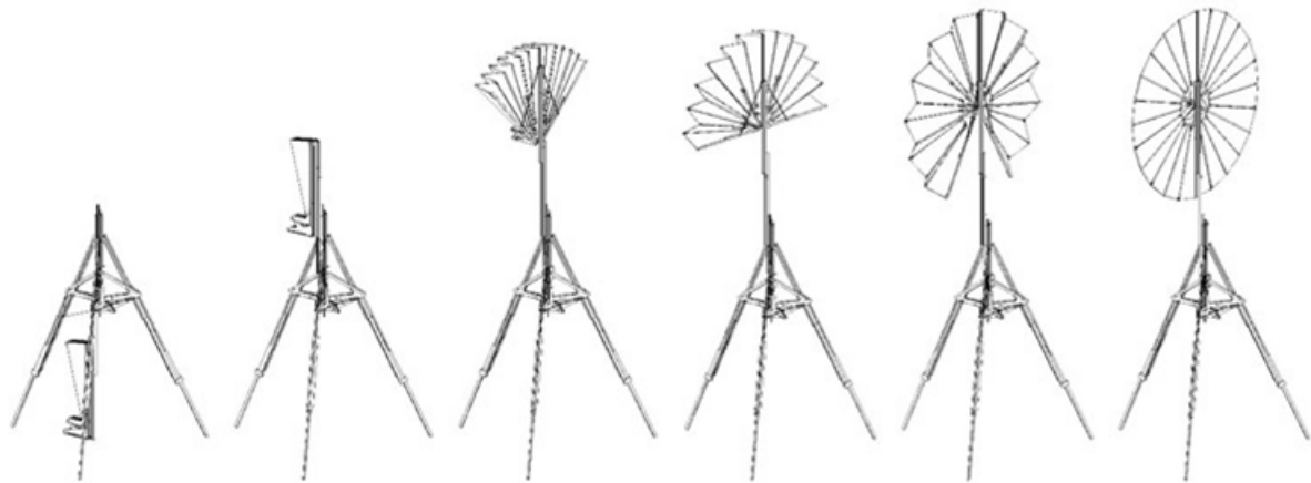
Figure 8. Sunflake lifting (left) Sunflake deploying (right)
