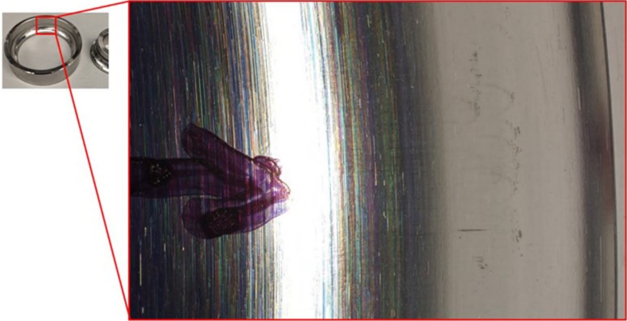
Figure 10. Bearing Outer Raceway at 50x Magnification
