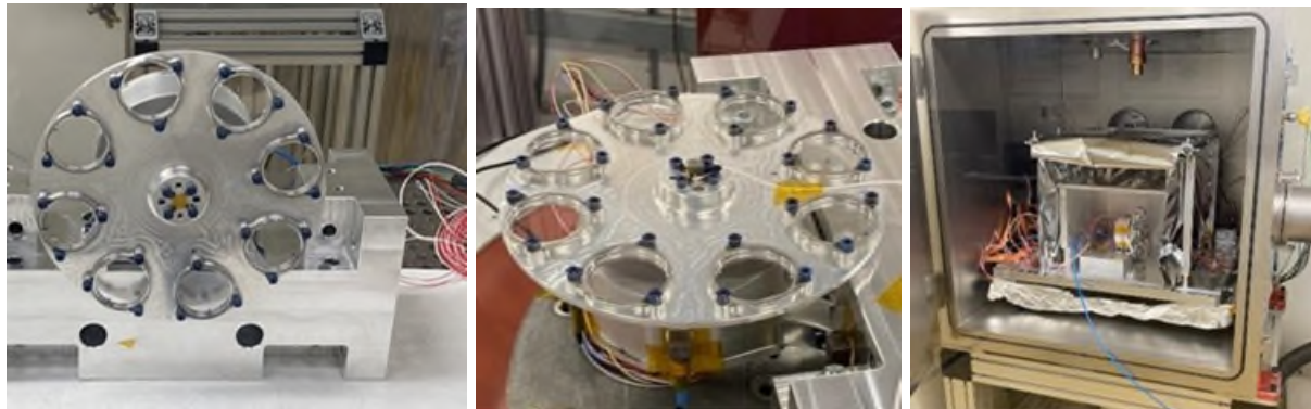
Figure 9. FWM breadboard as used for functional, vibration and TV & life testing
