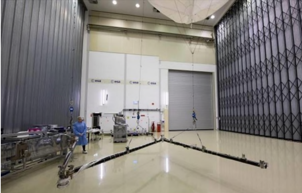
Figure 6 : Deployment of the MAGBOOM using helium balloons
