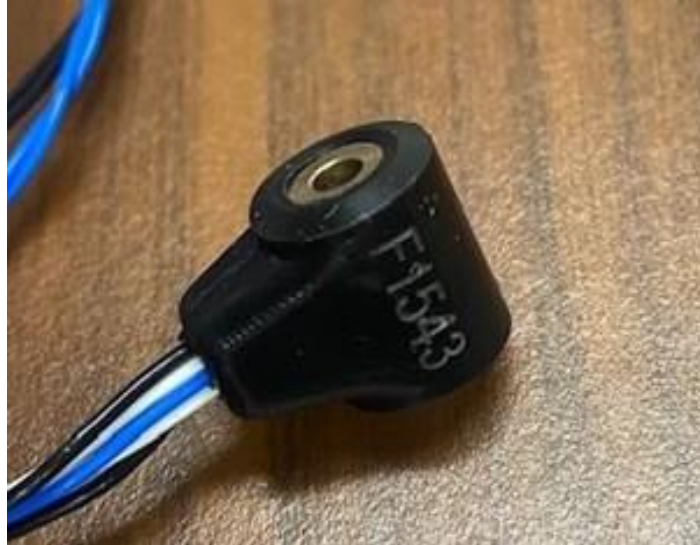
Figure 1. FD04 Frangibolt Actuator.
