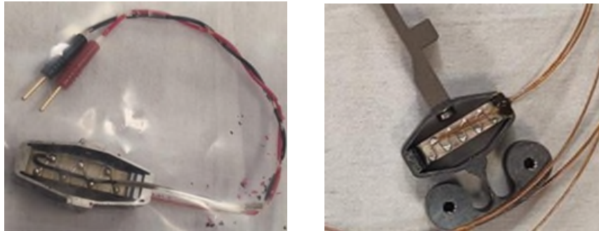
Figure 14. Pictures of two amplified actuators after exposure to 100 000 kRad left is using PTFE wire, right is Kapton wire
