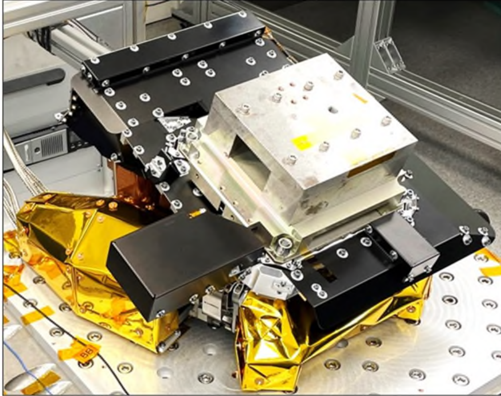
Figure 2. APPMAX2 in highly pre-loaded Launch Configuration (shown with Thruster Mass Dummy)
