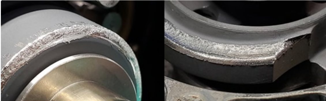
Figure 15. Galled surfaces seen after testing self-mated CPM 3V tool steel.
