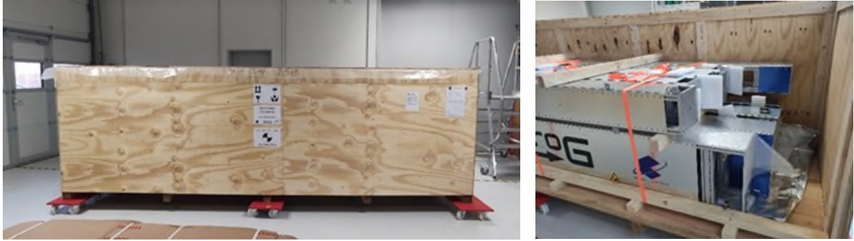
Figure 15: A modular ZeroG-system with four traverses is prepared for overseas shipping in one large box (left, ladder for scale). Right: With all Components neatly stacked, there would be room for another two traverses, allowing for six individual active gravity offloading suspension points at a stowed pitch of 30 mm.
