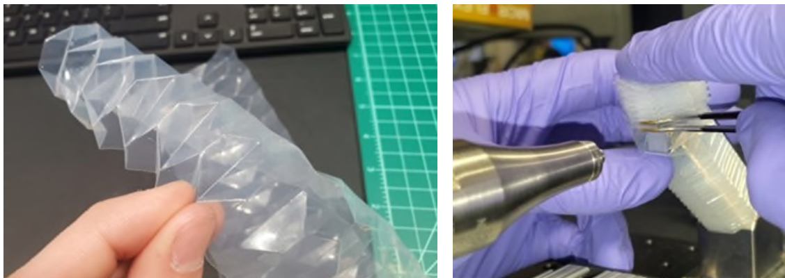
Figure 8. Folding (left) and ultrasonically welding (right) of ETFE bellows.
