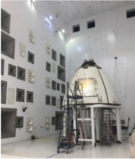
Figure 10 (Left). EDU LAS Hatch installed into LAS Ogive test assembly at NASA's Reverberant Acoustic Test Facility (RATF)
