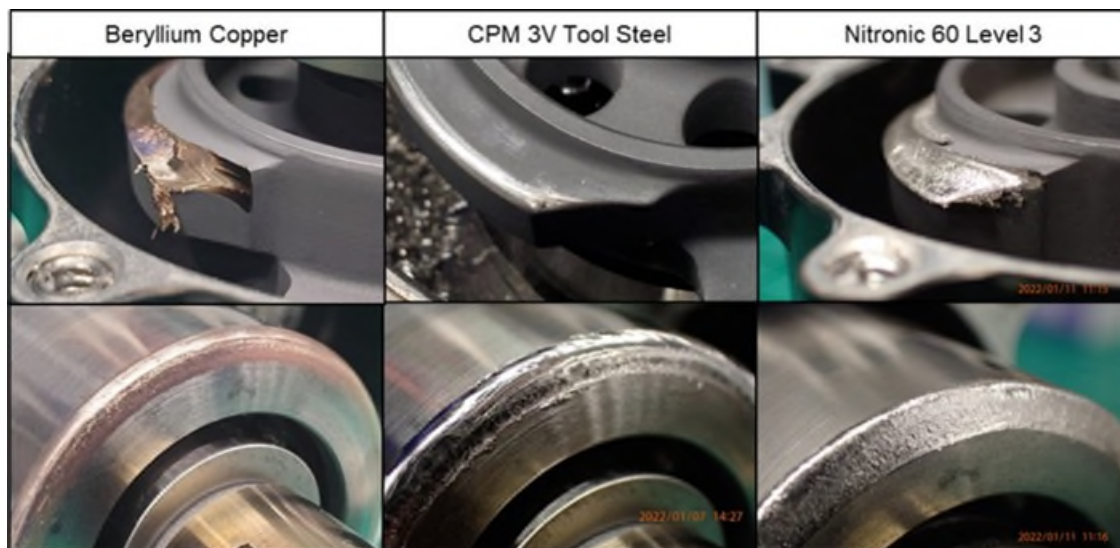
Figure 14. Condition of cams of various materials at top of ramp (top) after 80k cycles against a Vascomax C250 follower (bottom).
