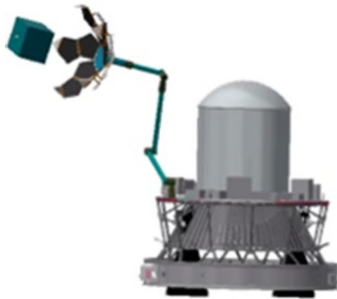
Figure 2. Robotic arm with engulfing end-effector used for capturing freely floating debris object
