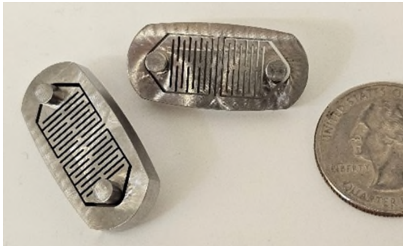
Figure 4. An example of multiple flexure blades in series to provide long stroke in a compact envelope. Note the integrated hard stop/load shunt. These linkages allowed 1 mm of linear motion and were used in an over-centering mechanism to provide reliable function without the need for adjustment. A small amount of discoloration can be seen because of excessive heat generated during the wire EDM process.
