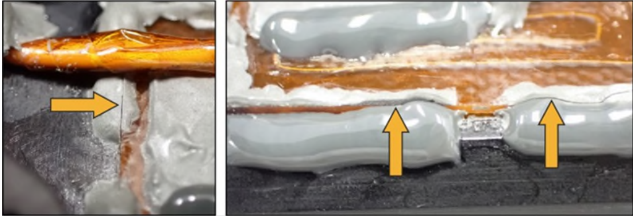
Figure 10. Lower Launch Lock Heater Staking Issues
