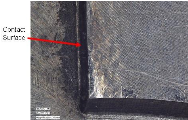
Figure 10. 150X Magnified Image of 0.25-mm Armature Teeth After Testing
