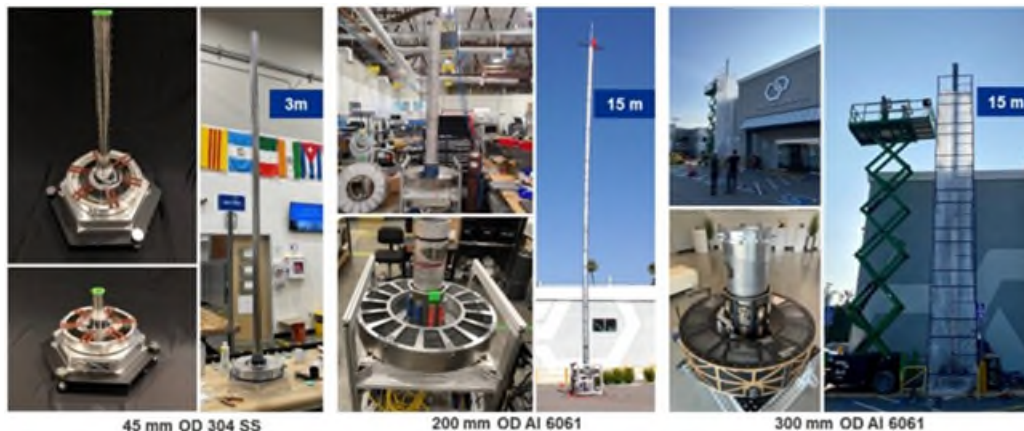
Figure 1. (left) DIABLO mechanism shown in stowed and deployed configuration with a diameter of 45 mm with a deployment length of 3 meters. (middle) DIABLO 200-mm diameter that can deploy up to 15 meters. (right) DIABLO 300-mm diameter that can carry 500-N payload on the tip.
