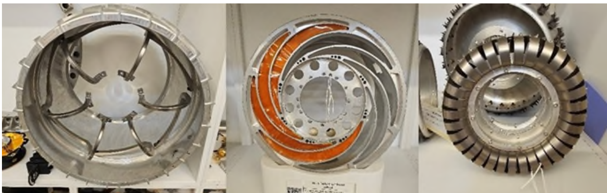
Figure 20. Three different Mars rover wheels, all using flexures to provide a simple suspension.
