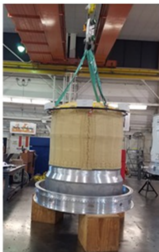
Figure 11 PASS Halo static load testing
