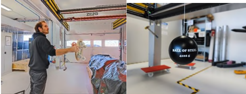
Figure 4: Several calibration masses were iterated. Despite the initial success with widely available rollerboards (left), we settled on the more standard ball of steel for calibration (right).
