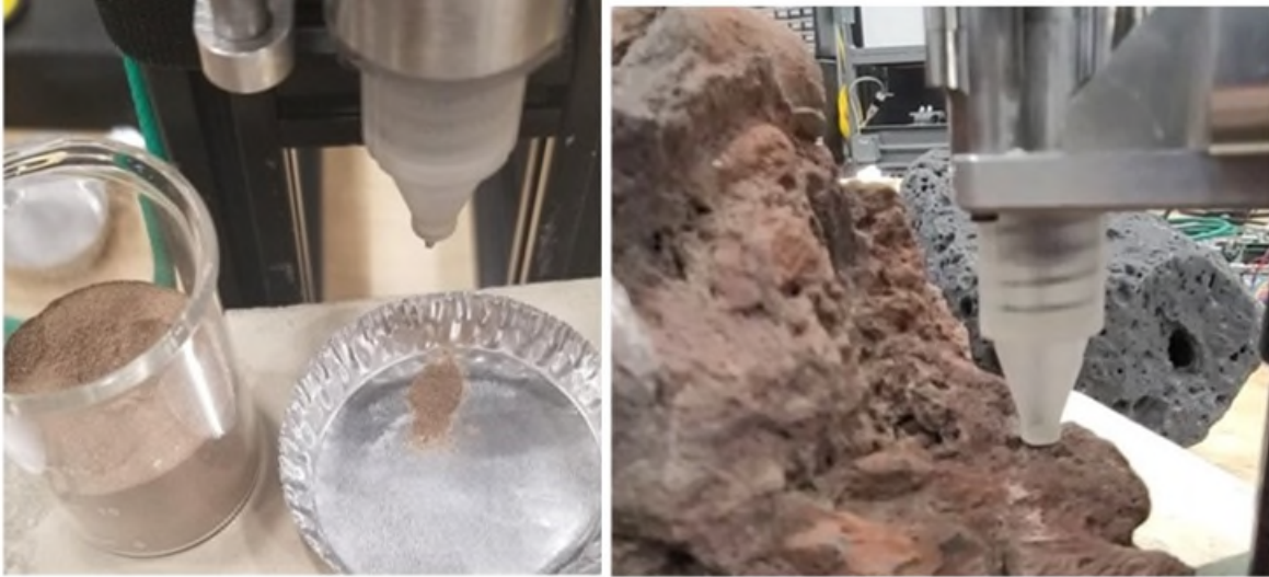
Figure 6. Simulant collected from a vial of unconsolidated material (left). Powder collection is possible on natural surfaces, but current system design is positioning dependent (right).
