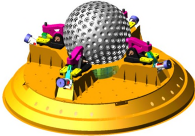
Figure 12. SSEP multibody model in preloaded configuration
