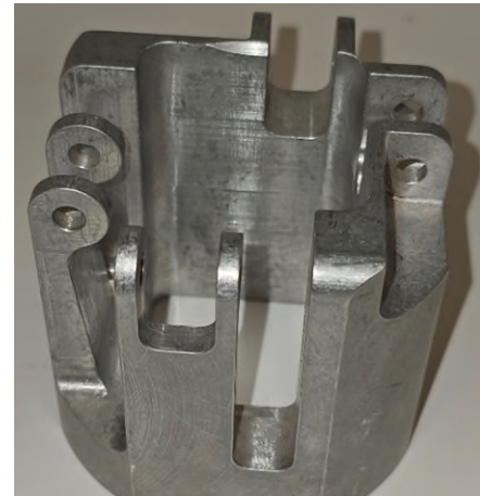
Figure 22. A flexured rod guide. The extremely low cycle requirement allowed the use of aluminum 7075 for this part.
