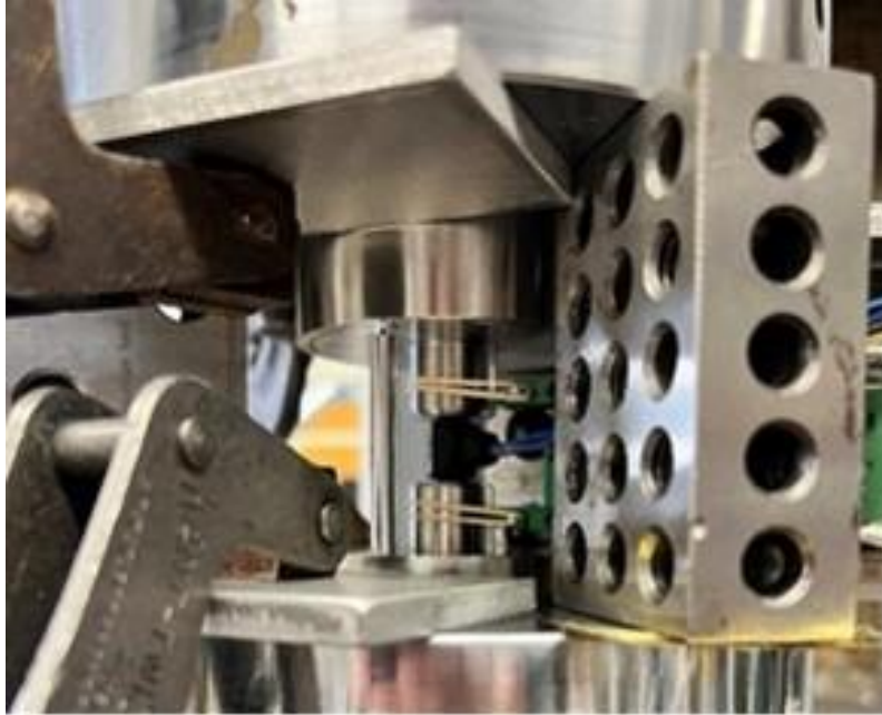
Figure 7. Instron top platen lowered onto the assembly with spacer blocks (shimmed gauge blocks with holes) and guide plates (metal plates clamped onto Instron to prevent slipping)
