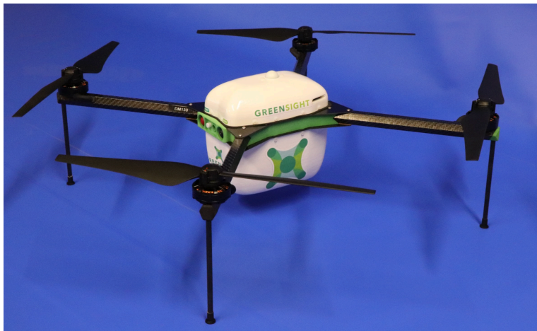
Figure 1: Dreamer UAS. The GreenSight Dreamer vehicle uses Ardupilot autopilot software [6] and GreenSight Ultrablue flight controller with architecture similar to the Pixhawk [7].
