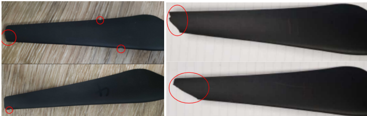
Figure 31: Examples of blade minor (left) and blade major (right) damage.
