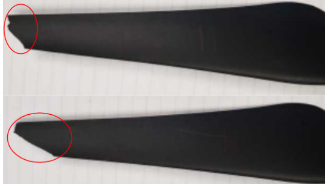
Figure 5: Major blade damage,
