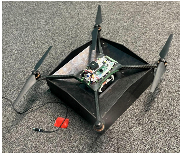
Figure 3: Instrumented Dreamer in two versions of the preflight testing cradle (clamped and unclamped) used during data gathering,
