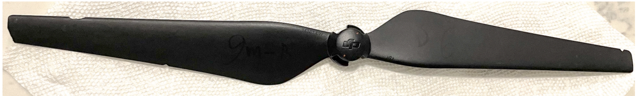
Figure 6: Minor blade damage.
