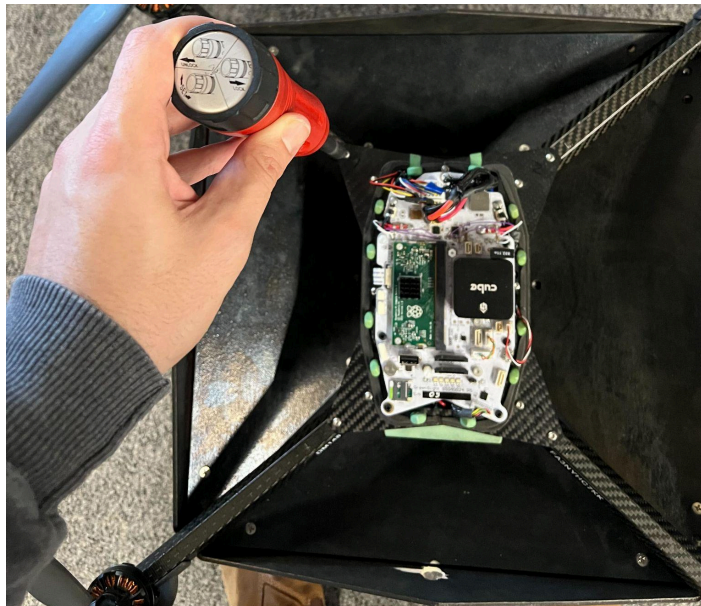
Figure 7: Uncovered Dreamer UAS outer arm screw being adjusted with a torque wrench.
