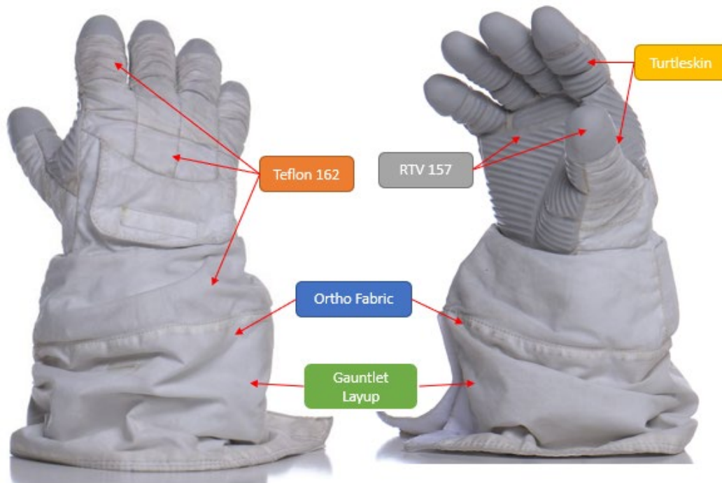
Figure 5. Phase VI TMG Fabric and Ply-up Locations. Teflon T-162 is located on the outside of the hand back and wrist portion of the glove, RTV 157 is the compound used to form the palm and finger pads, Ortho Fabric is located in the wrist and is also the outer fabric of the EMU, Turtleskin is used as a cut resistant layer on the fingers and palms. The glove gauntlet is a ply-up of fabric (Teflon, multilayered insulation (MLI), Ortho) that covers the suit lower arm.
