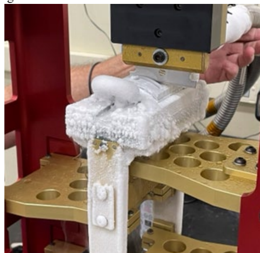
Figure 7. Frost Accumulation During Data Collection. The specimen holder and surrounding components collected more than expected frost during testing but did not affect the function of the machine.
