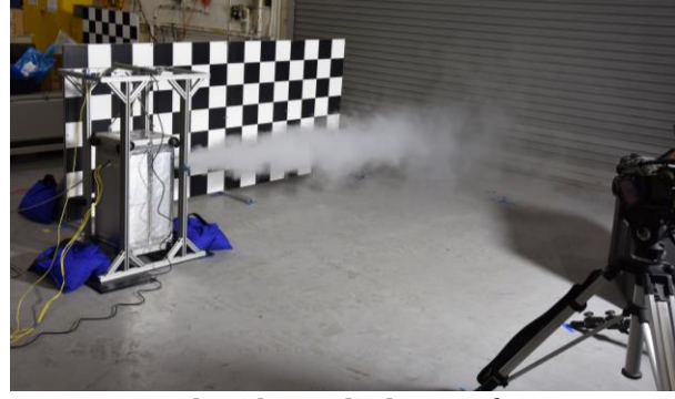
Figure 7. Right-side-up discharge of C-100 HFC-227ea PFE.
