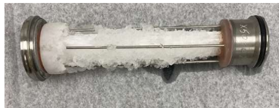
Figure 18. Water frozen along external length of Cartridge 4 following full wet-out.
