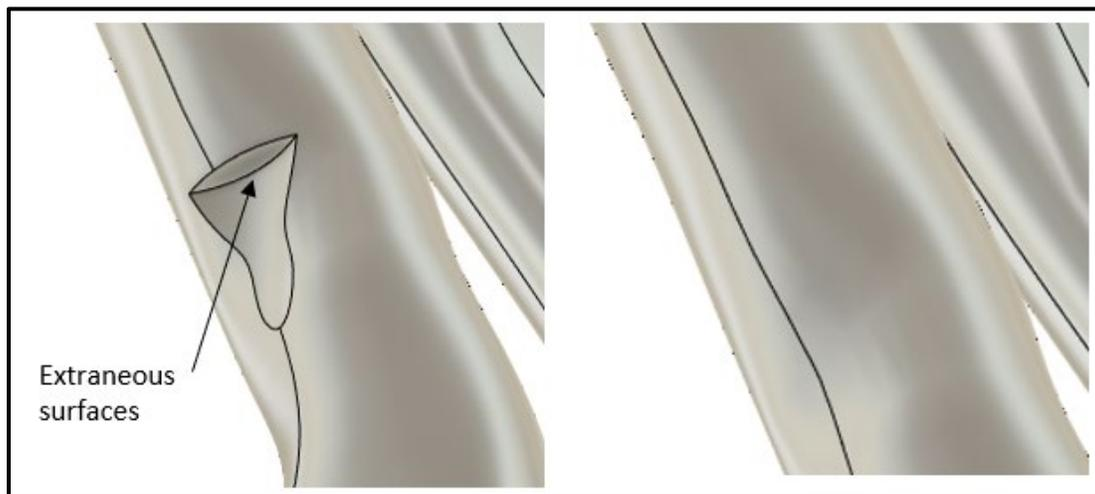
*Figure 4-1. Extraneous surfaces caused by obstacle cuts can be deleted to clean up the CAD geometry.*
