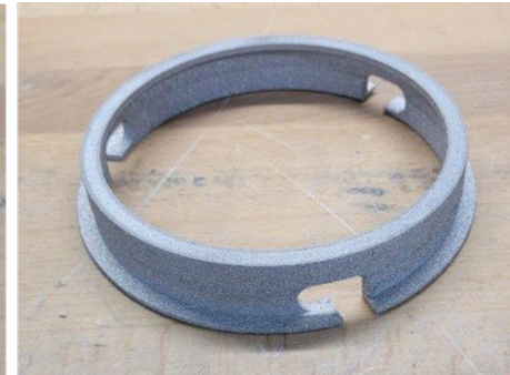
Space Suit Wrist Disconnect manufactured by FabLab. Image courtesy of Techshot a Redwire company.
