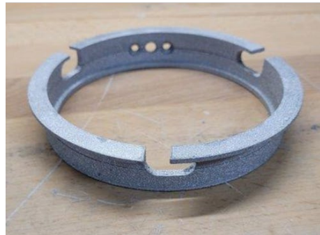
Space Suit Wrist Disconnect manufactured by FabLab. Image courtesy of Techshot a Redwire company.
