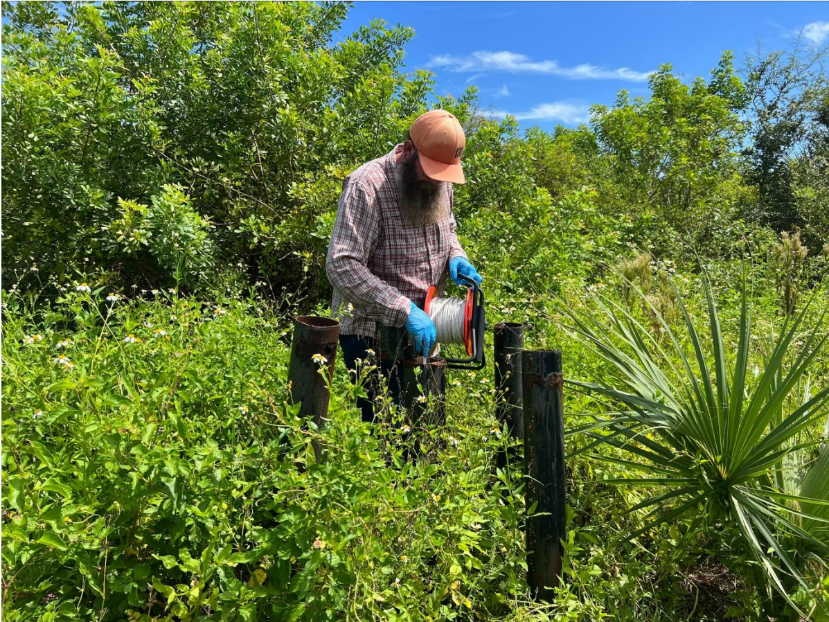
3: Collecting static water level reading at monitoring well IW0029ID. (Photo was taken facing east.)
