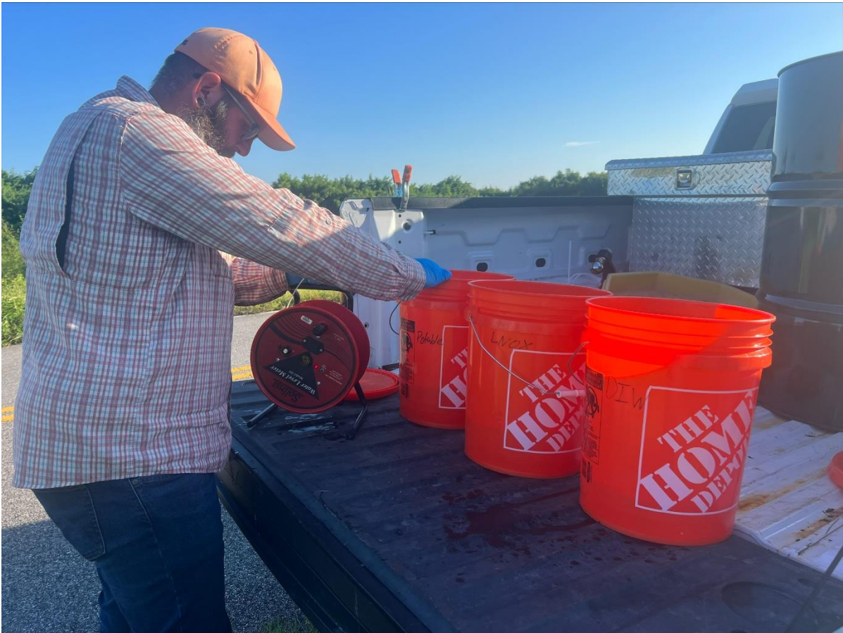
4: Deconning static water level meter with potable water, Luminox wash, and DI water.
