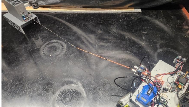
Figure 7. Microbase with tether and boom attached to reel mechanism.
