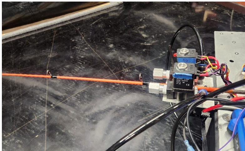
Figure 8. Close up on tether boom and articulated thruster pod.
