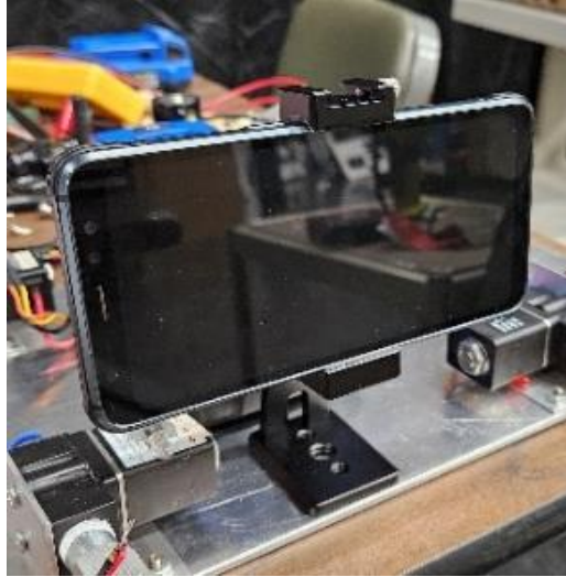
Figure 13. Ruggedized Samsung smartphone in adjustable mount attached to the electronics deck.
