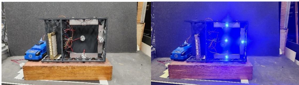
Figure 11 and 12. LED target assembly, powered by a 24V battery to light four high-intensity blue LEDs.
