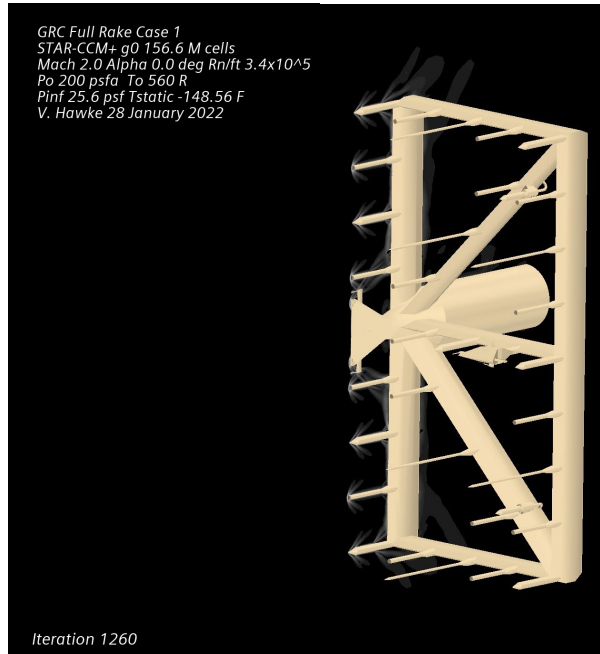
Figure 8: CFD simulation of 10x10 SWT Characterization Array for drag estimation at Mach 2.0, Reynolds number 0.34 \times 10^6 per foot.
