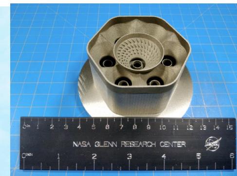
Turbine engine combustor (fuel-air mixer) 3-D printed from GRX-810
