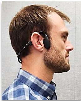
Figure 3. Photo of NASA engineering test subject modeling Code Red Zero-M bone conduction headphones.
