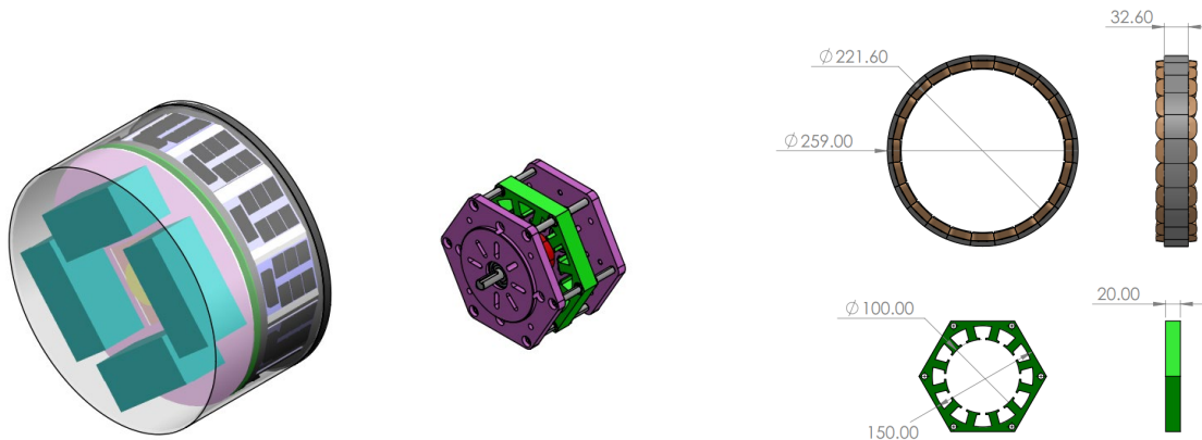
Figure 3-5.—To-scale comparisons of the developed quadrotor machine and identified sample design: (a) housing integration; and (b) stator dimensions in millimeters. Note the final demonstrator dimensions vary from those shared above.
