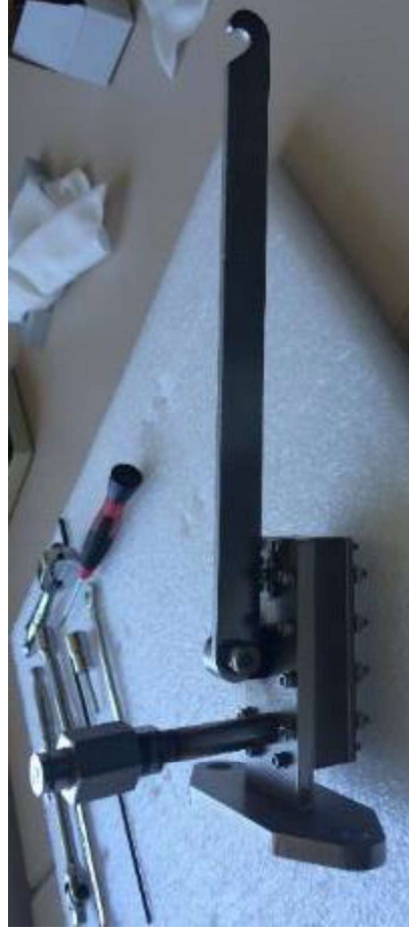
NASA Designed Loading Fixture for Exposure to LMP-103S Propellant – NASA New Technology Report (1461267027)
