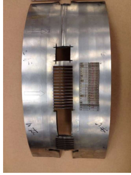
Specimen cut using Wire EDM
